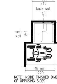
FIGURE 608.2.1 TRANSFER TYPE SHOWER COMPARTMENT SIZE AND CLEARANCE
