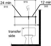
FIGURE 604.5.1 SIDE WALL GRAB BAR AT WATER CLOSEFFIGURE 604.5.2 REAR WALL GRAB BAR AT WATER CLOSETS
