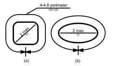
FIGURE 609.2.2 GRAB BAR NON-CIRCULAR CROSS SECTION
