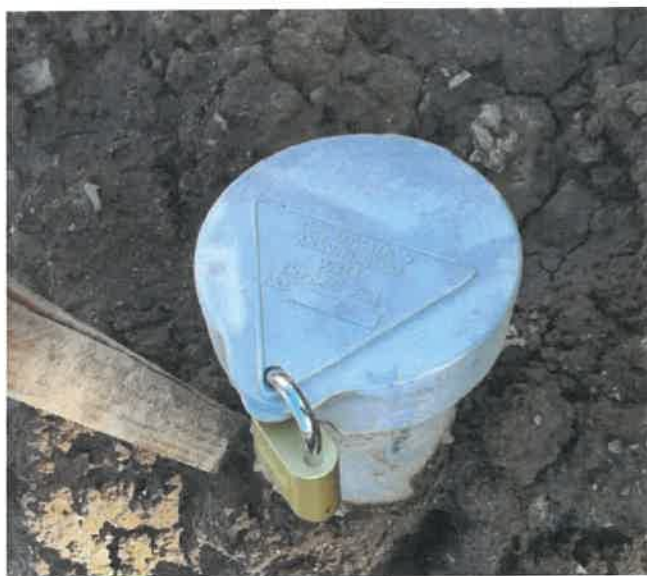
Figure 7: Photograph of closed drill hole capped and locked on drill pad 1 from the Amanita 2020 drilling. This drill hole had standing water and could be an alternative water source for drilling during 2026-2028 RC drilling.
