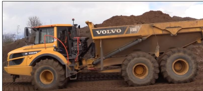
Figure 2-19. Typical Project Haul Truck (Volvo A30G)
