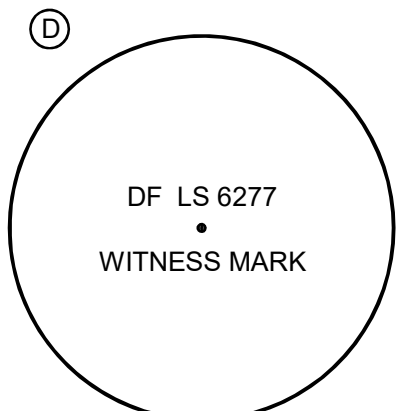
1.25" RED PLASTIC CAP SECONDARY MONUMENT RECOVERED THIS SURVEY GOOD CONDITION
