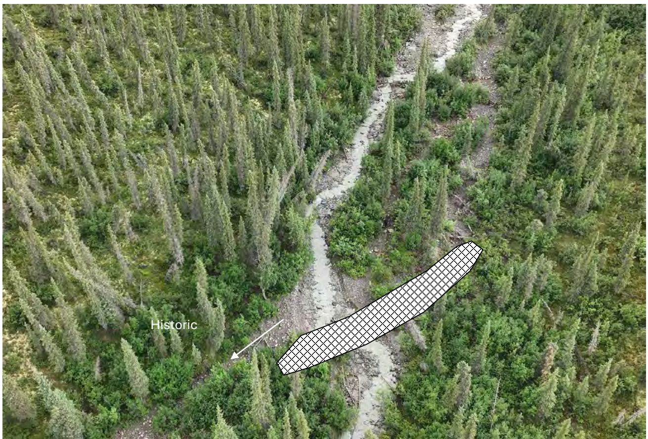
Figure 6. Recommended Dike Layout – spanning the dike across the entire channel will capture any flow that enters the secondary channel.
