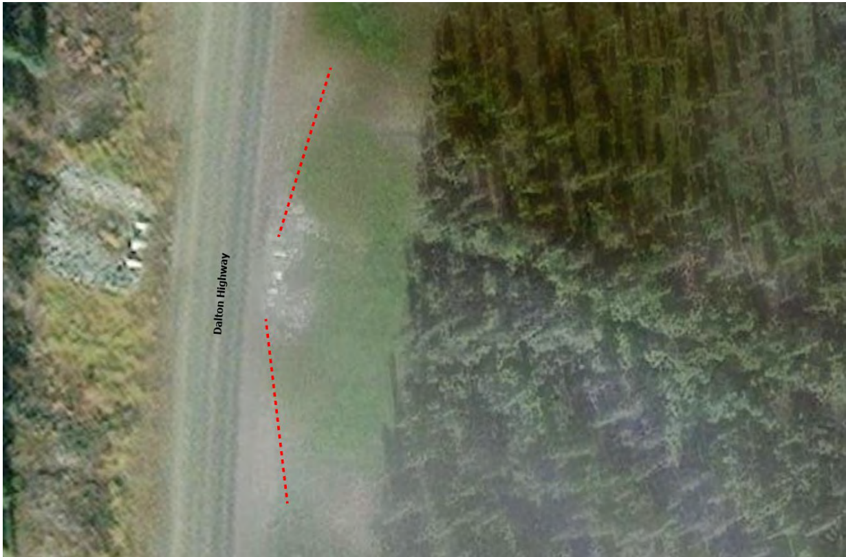
Figure 8. Recommended location of guide berms using removed material from berm blocking abandoned channel.
