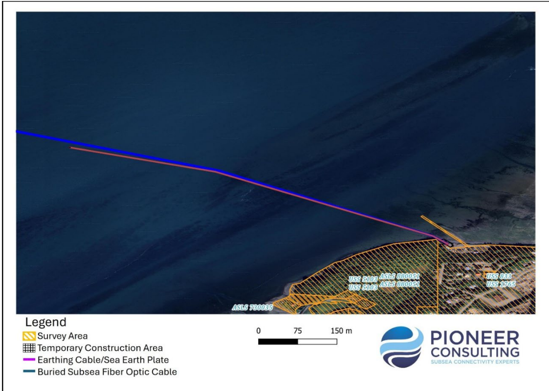
Figure 6: FISH in SEAK Cordova Landing with Earthing Cable to Sea Earth Plate.
