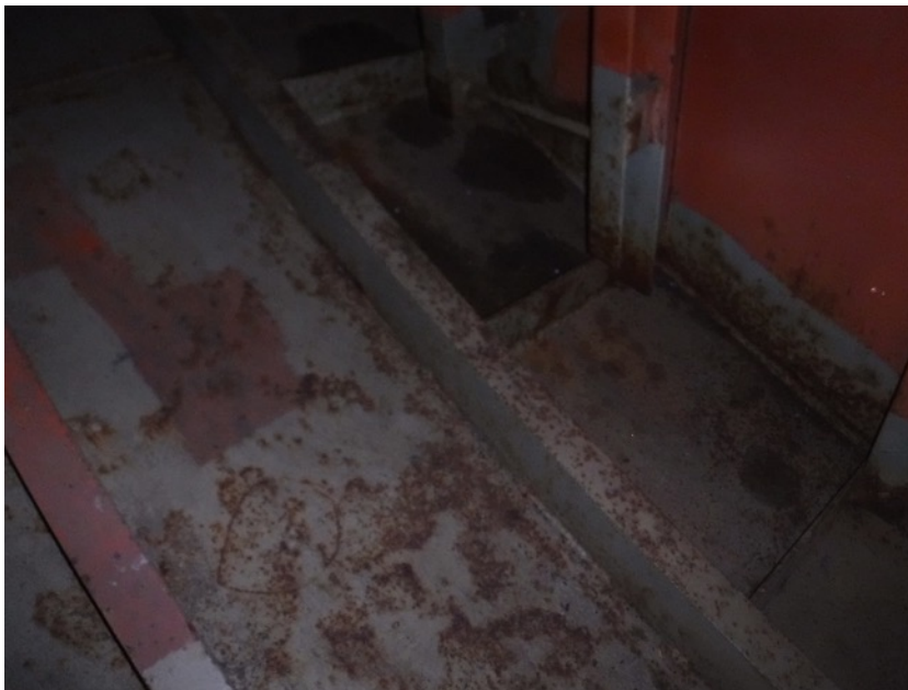
Photo 41: Minor Corrosion in Lower Section of No. 10 Port Void
