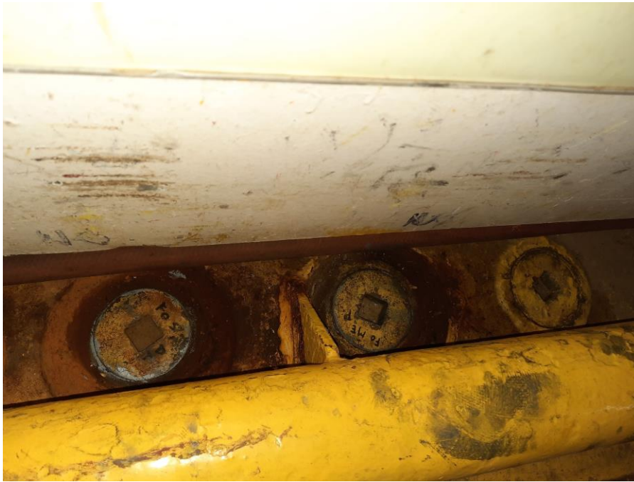
Figure 9 Worn sounding tube caps
