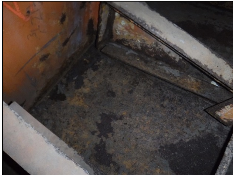
Photo 50: Corrosion in Lower Aft Section of No. 10 Port Void
