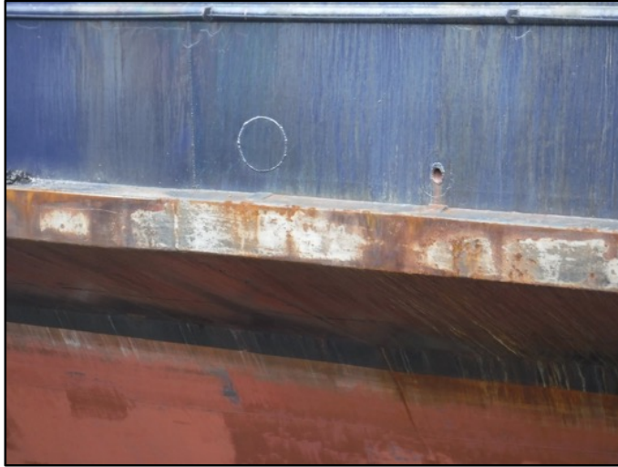
Photo 65: Rust Bleed Under Vents & Drains
