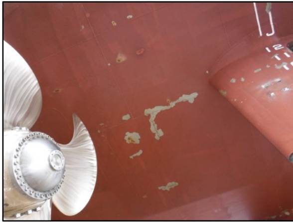
Photo 68: AF Delamination Spots Near Stern
