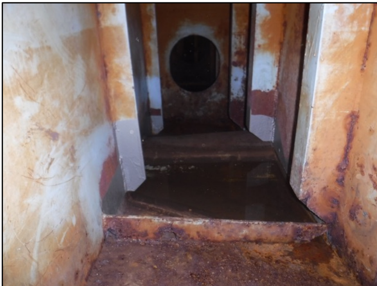
Photo 52: Corrosion on Deck of Cross Flood
