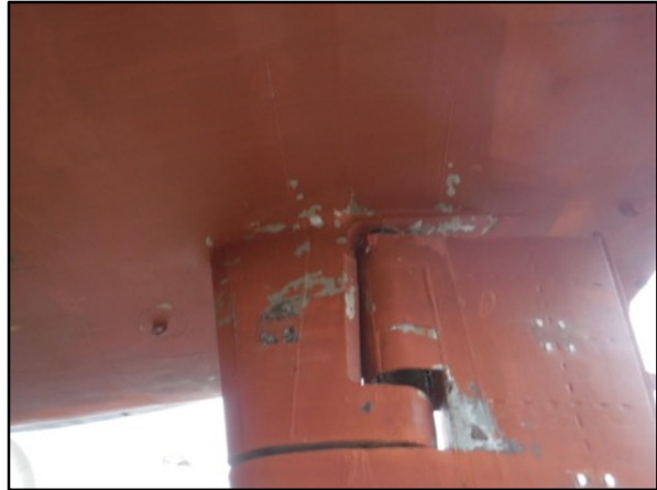
Photo 69: AF Delamination Spots on Rudders
