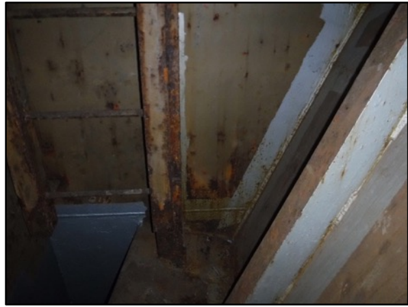
Photo 6: Corrosion on Aft Bulkhead
