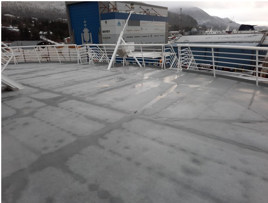
Figure 8 Dishing on aft Boat Deck
