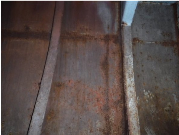
Photo 50: Corrosion in Lower Aft Section of No. 10 Port Void
