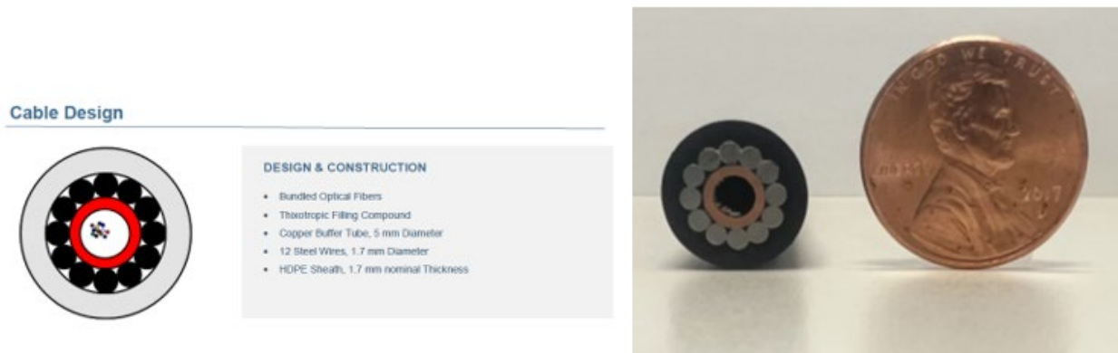
Figure 4: Fiber optic cable specifications.
