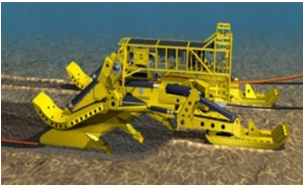
Figure 8: Submarine Cable Plow
