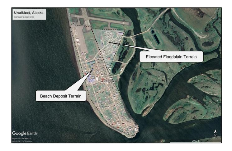
The terrain units are predicated primarily on our interpretation of undisturbed in-place soil and ground thermal states from the geotechnical data we reviewed for this submittal. Surface and near surface fill and development is expected to mask the underlying in-place soils particularly along roadways, airstrips, and other developments.
