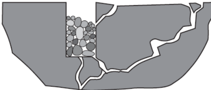
Figure 13-2 Incompressible Causing Spalling at a Joint or Crack
