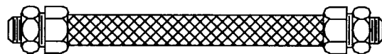
14. FLAME RESISTANT FLEXIBLE FUEL HOSE (2) FURNISHED BY ENGINE MANUFACTURER FOR SUPPLY AND RETURN LINES
