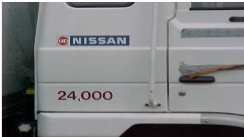
Some vehicles will show the GVWR of the vehicle on the door panel
