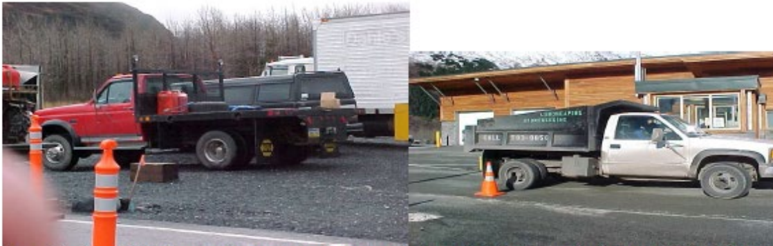
Generally these 3500 Series pickups with dually rear ends & modified beds usually have a GVWR of 12,000 or more.
