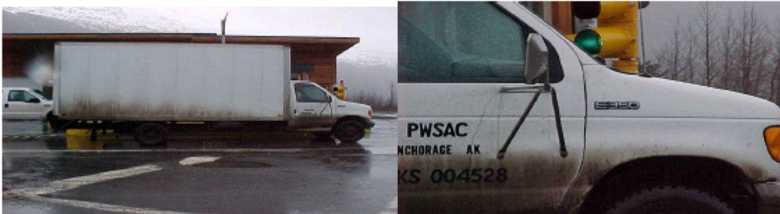
DOT number is a good indication that this vehicle's GVWR is over 12,000lbs.
