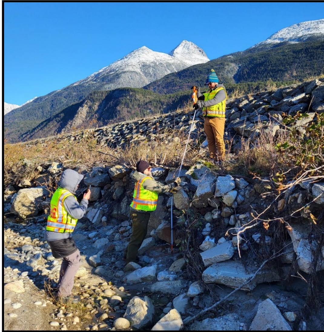
Figure 7 - Erosion along toe where airport modification was complete in 2001. Measured 5 feet of scour in this location.
