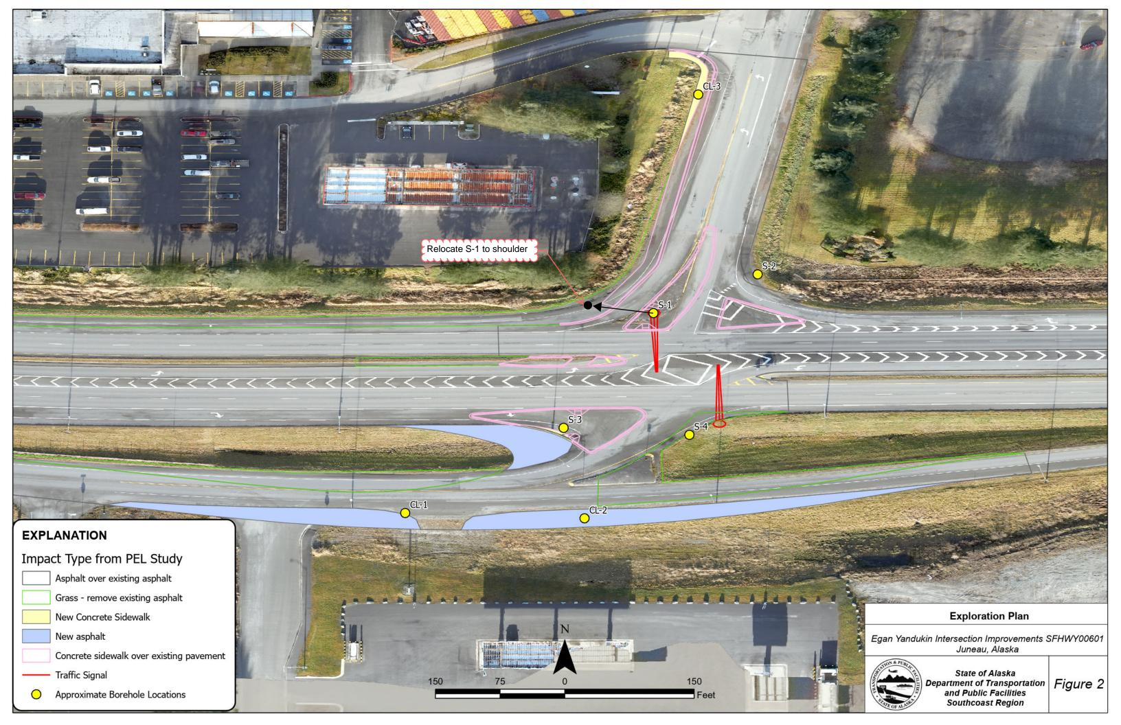
Work Zone A & B **Yandukin Intersection- Lane Shift Example Temporary Traffic Control Plan** For Test Hole Location: CL-3, S-1, S-2
