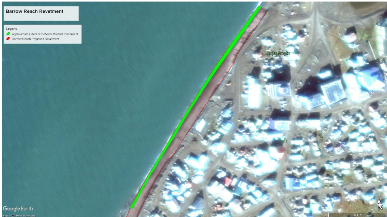
Figure 4. Approximate In-Water Extent of Revetment Construction
