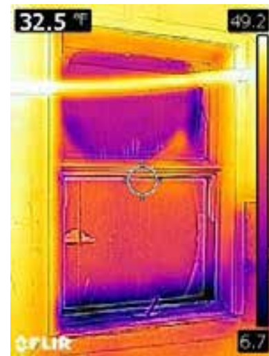
Figure 2: Thermal Images of a Broken Window and a Boarded Window in the Water Treatment Plant
