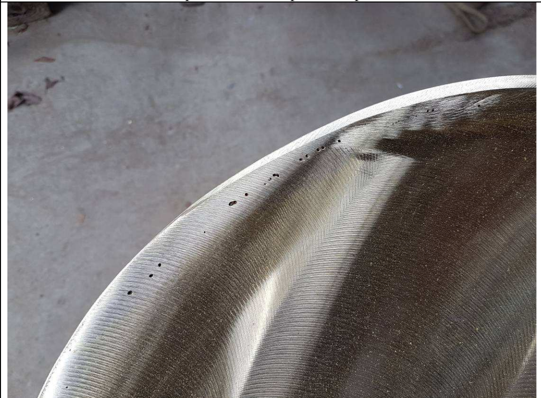
Photo of blade edge after sanding, showing material difference
