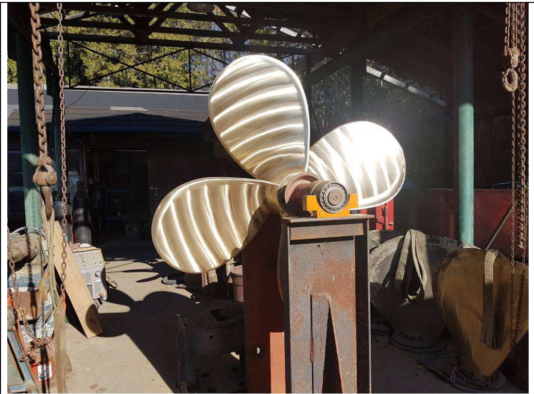
Port, LH propeller on balancing stand
