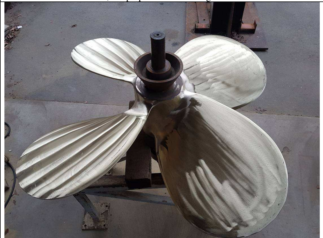
Sanding suction face of starboard propeller
