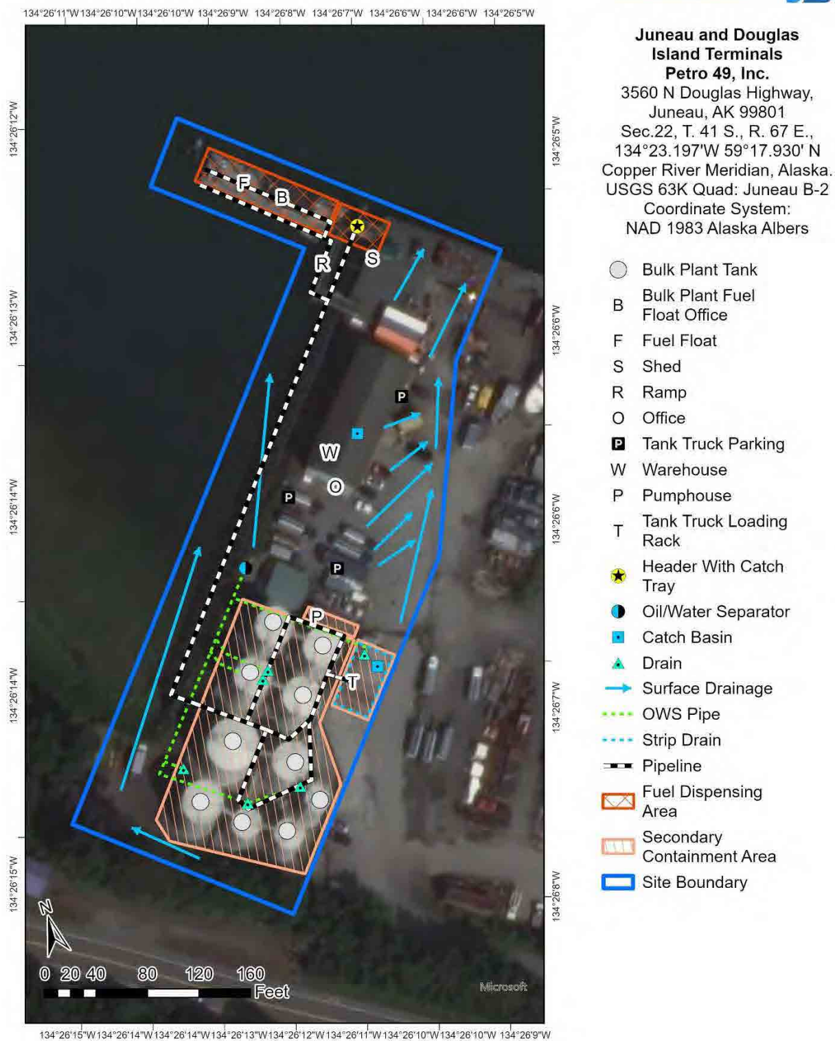
Figure 1.8-15 Douglas Island Terminal Site Drainage
