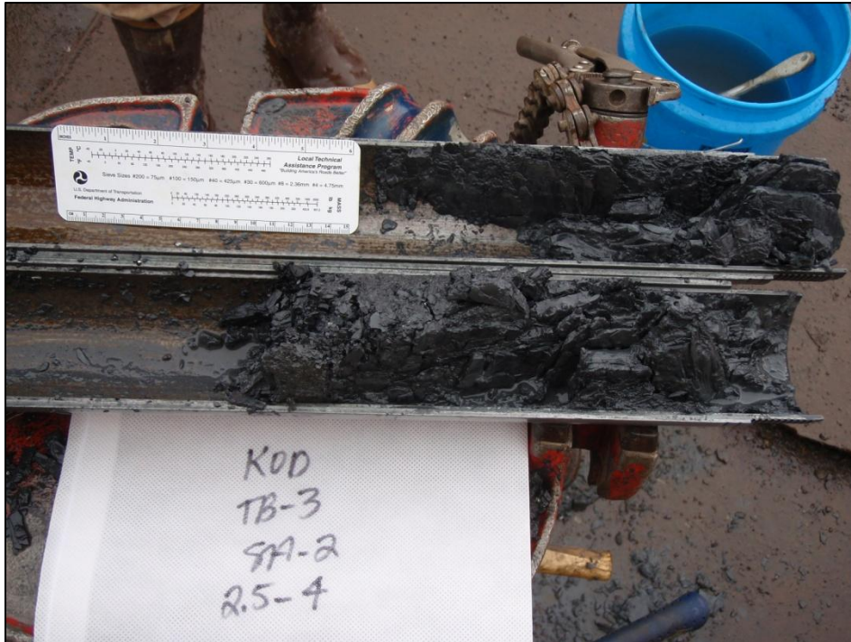
Photograph No.2: Sample of slightly weathered bedrock from test boring AP-149 taken between 2.5 and 4.0 feet below the mudline.
