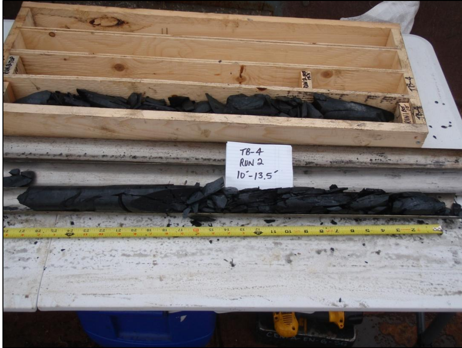
Photograph No.3: Sample of bedrock from test boring AP-150 taken between 10.0 to 13.5 feet below the mudline. Reported ASTM D 6032 Rock Quality Designation (RQD) = 0.
