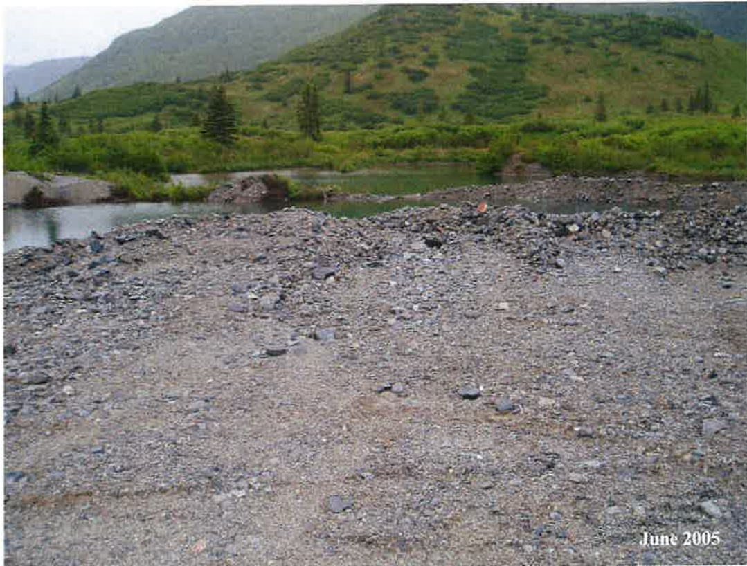
MP 6 Pit - Existing gravel pit at MP 6. Owned by CIRI. Collected a sample from the edge of the pond at berm/stockpile. The material is mined from below water. Groundwater is only 2 ft below ground.
