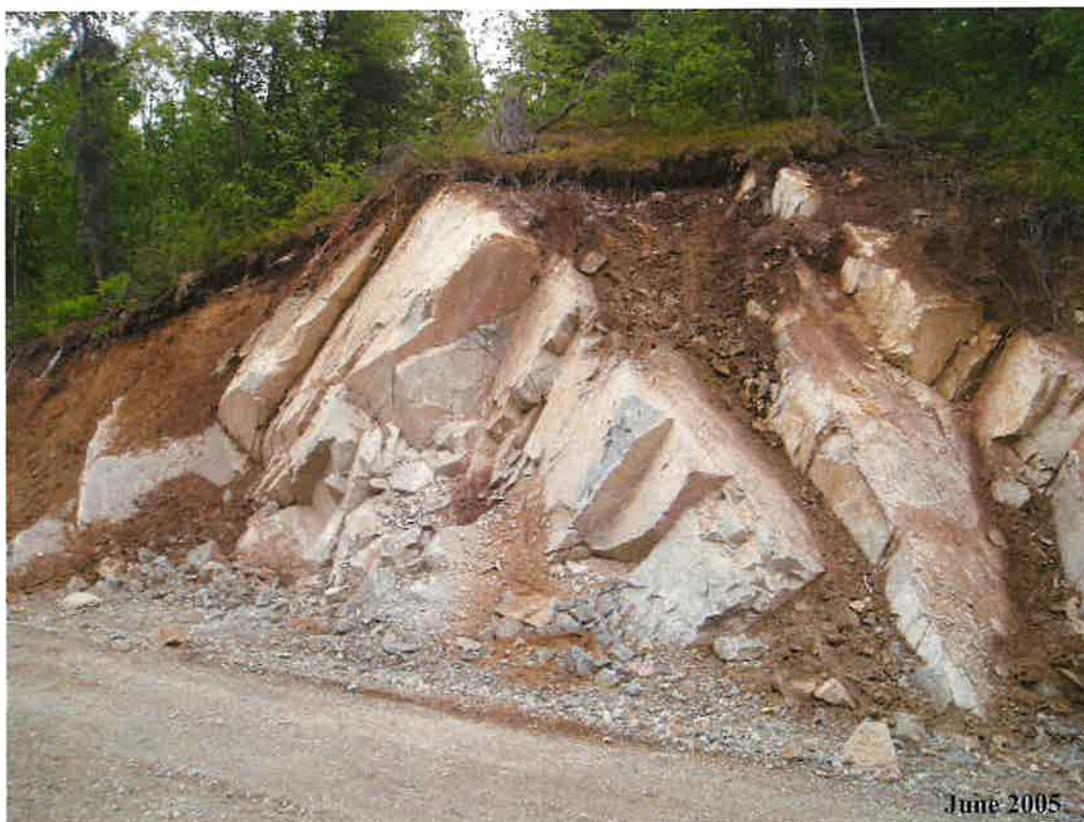
MP 13.4 - Bedrock exposed in the cut. Wide spaced joint pattern in this cut makes it a good prospect for a rip rap source.
