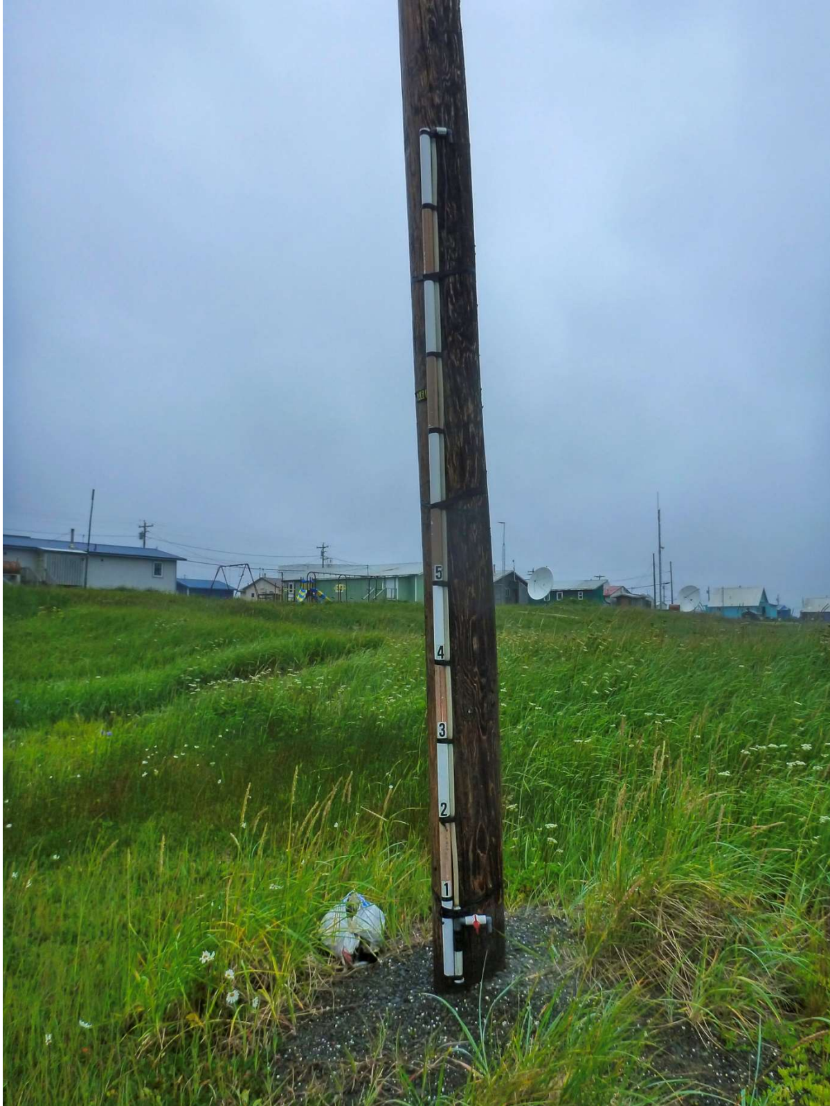
Figure 10: Tide gauge adjacent to the winter water source pump house. Records for the gauge were not available.
