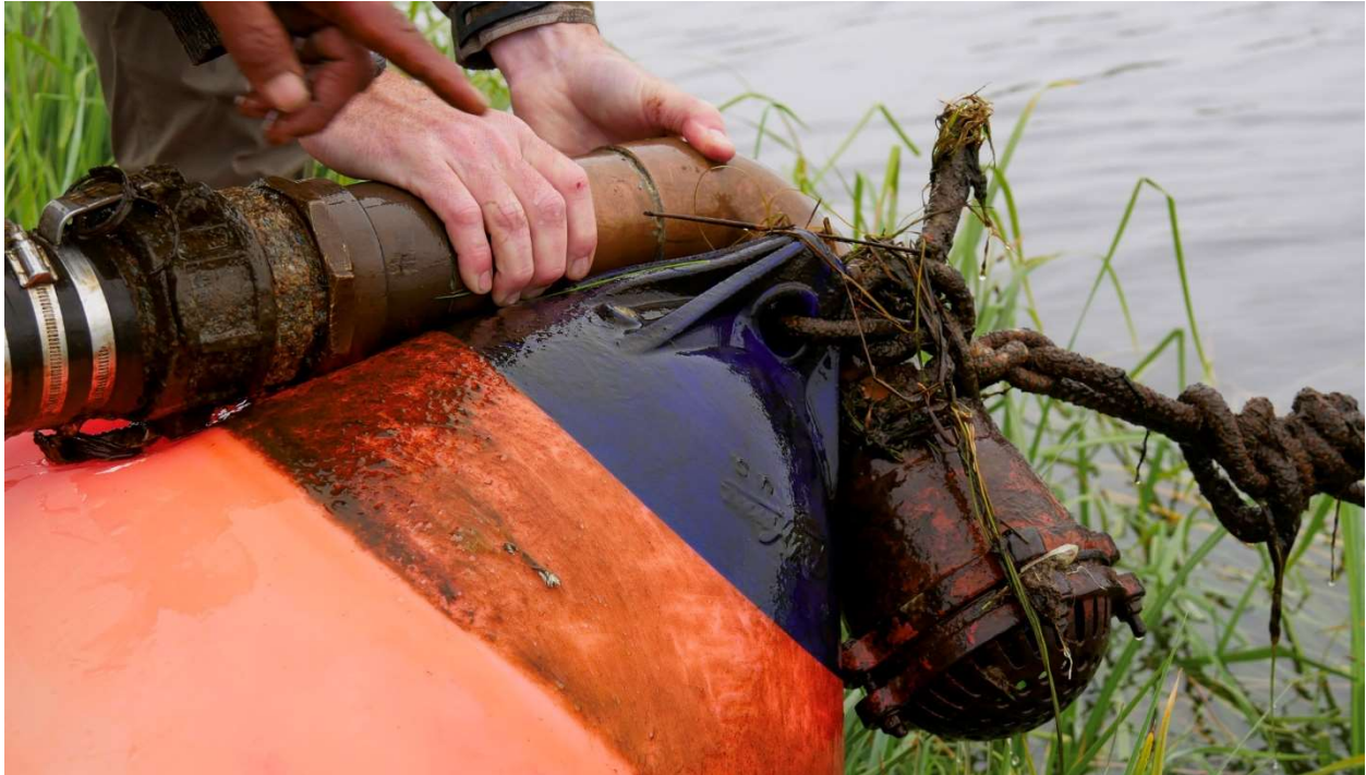
Figure 3: Water source intake foot valve. The same intake foot valve is used for the summer and winter intakes (pictured at the summer water source).
