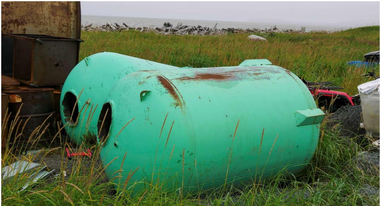
Figure 32: Previous filters, 4 feet diameter by 6 feet tall.
