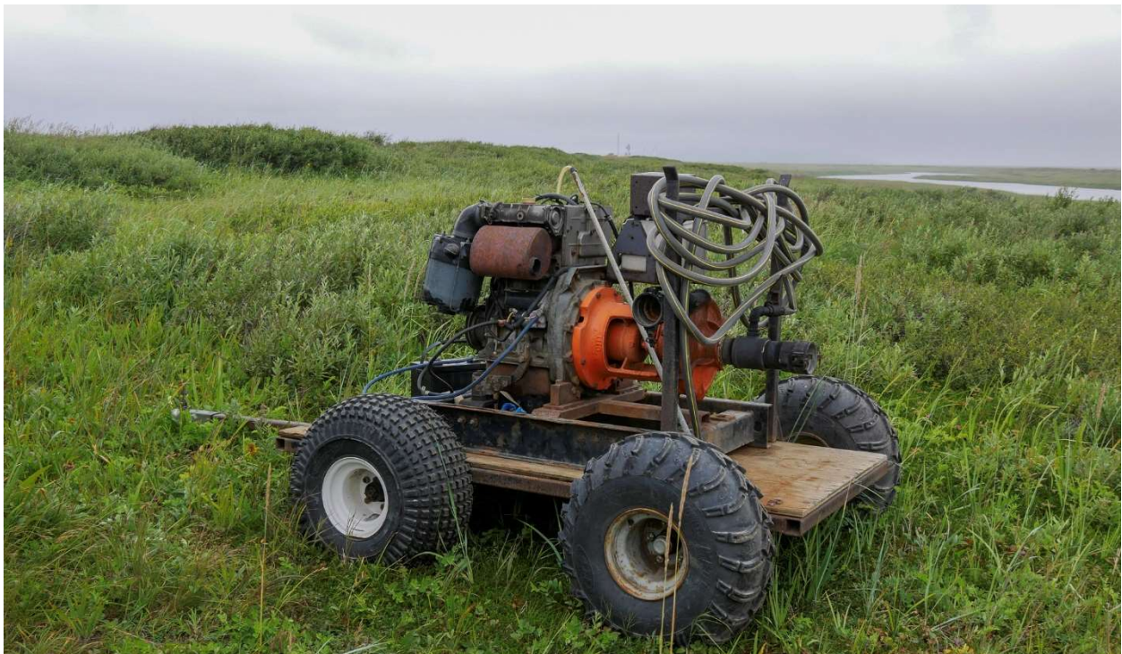
Figure 41: Diesel engine powered pump located at the summer water supply point.
