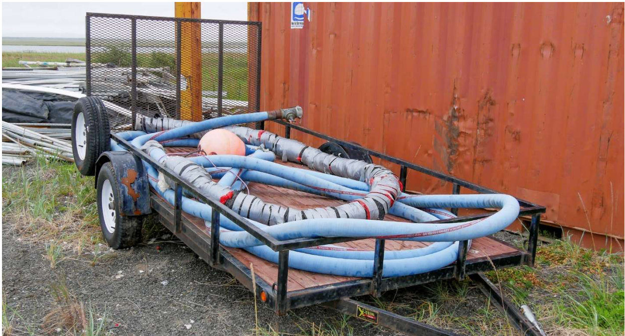
Figure 4: Trailer with hoses used at the winter water source for fill operations (roughly once every six weeks). The 100 foot long 3 inch diameter hose (blue) connects to the foot valve (pictured in Figure 3) and runs from a hole in the ice to the pump house where it connects to the pump suction. The 20 foot long 4 inch diameter discharge hose (wrapped with duct tape to secure heat trace and homemade insulation) runs from the pump discharge to the Winter Raw Water pipe connection point (photos provided on subsequent pages).
