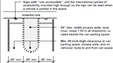
96" min. width access aisle, level (max. slope 1:50 in all directions), located beside the van parking space
