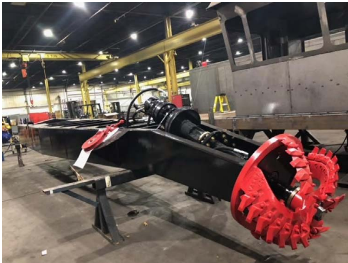
Figure 5-7. Cutterhead and ladder under construction
