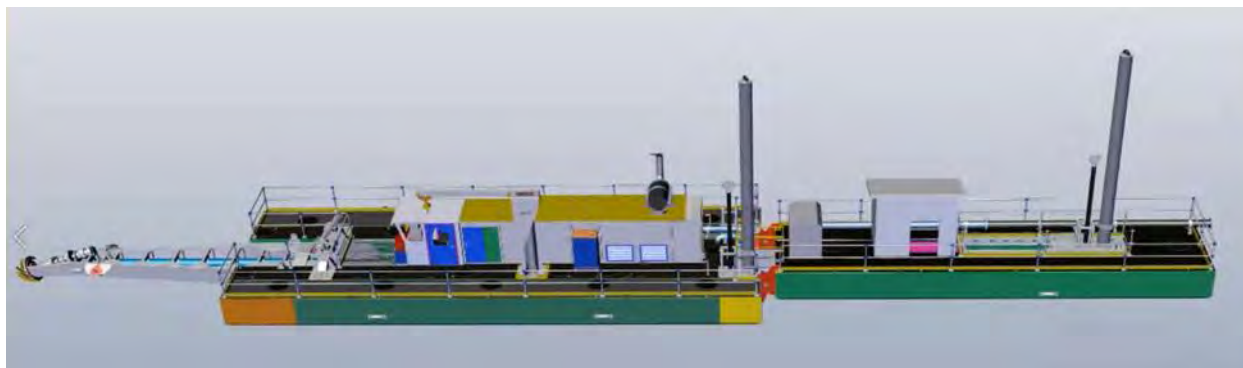
Figure 5-10. Complete assembled cutterhead dredge and idler float
