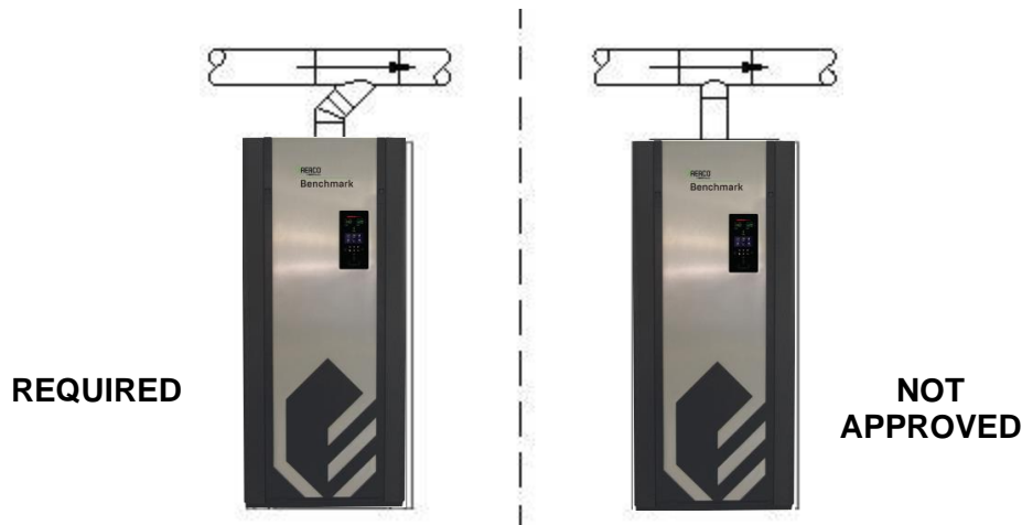
Figure 11a: Required Connections to Common Vent Breeching
