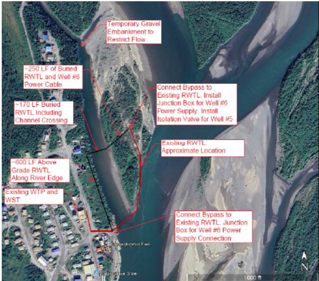
Figure 4: Overview of Emergency Bypass Alignment (in black)
