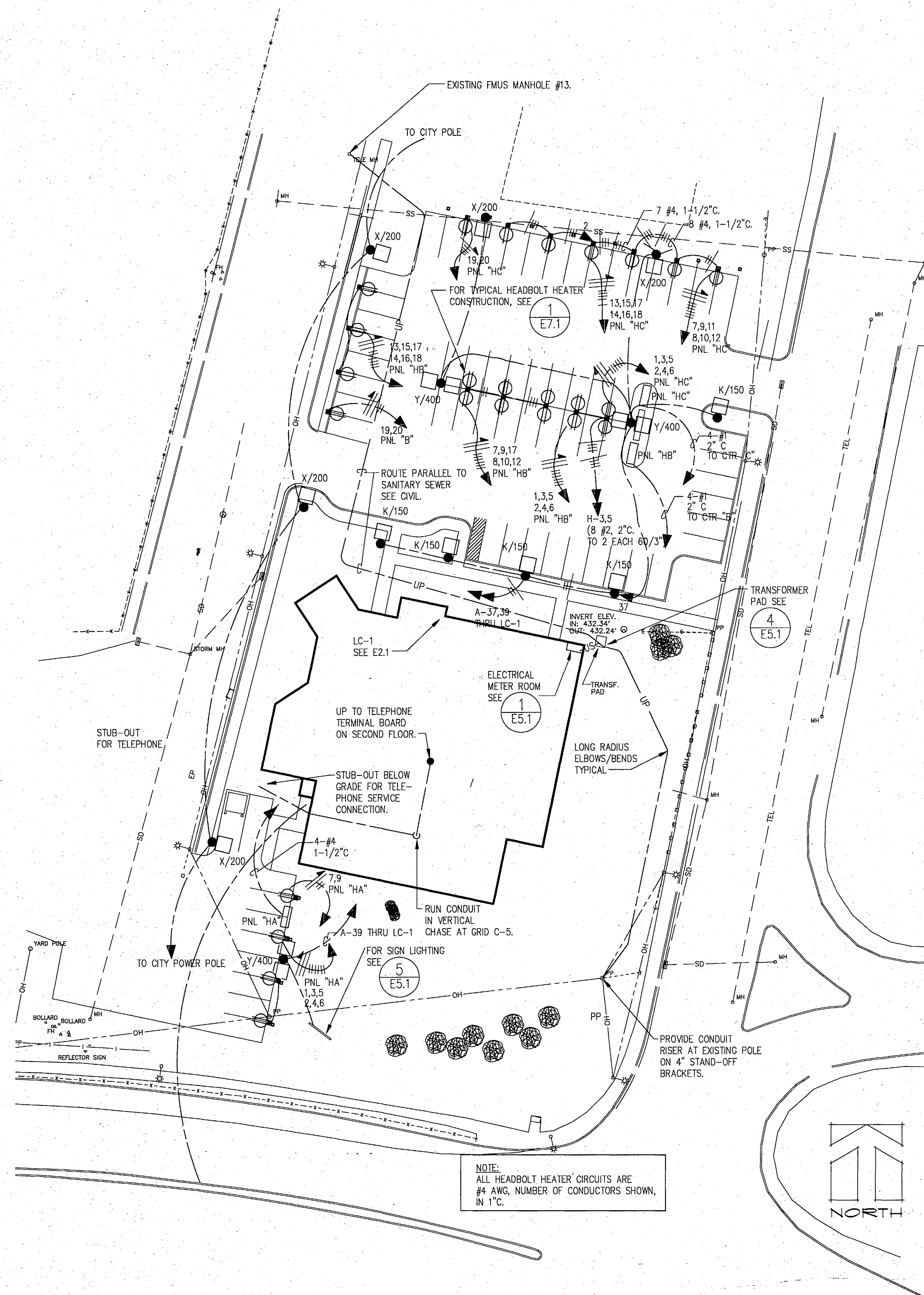
ELECTRICAL SITE PLAN - NEW WORK 1"=30'-0"
