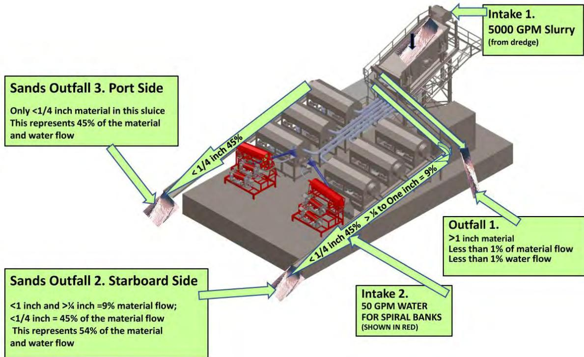
The 1" to ¼" material from the lower screen is diverted into a 24" chute connecting to the starboard side nugget sluice, which is labeled *Sands Outfall 2* in Figure 5-12. The 1" to ¼" gravel product will constitute approximately 9% of the total solids volume out of *Sands Outfall 2*.
