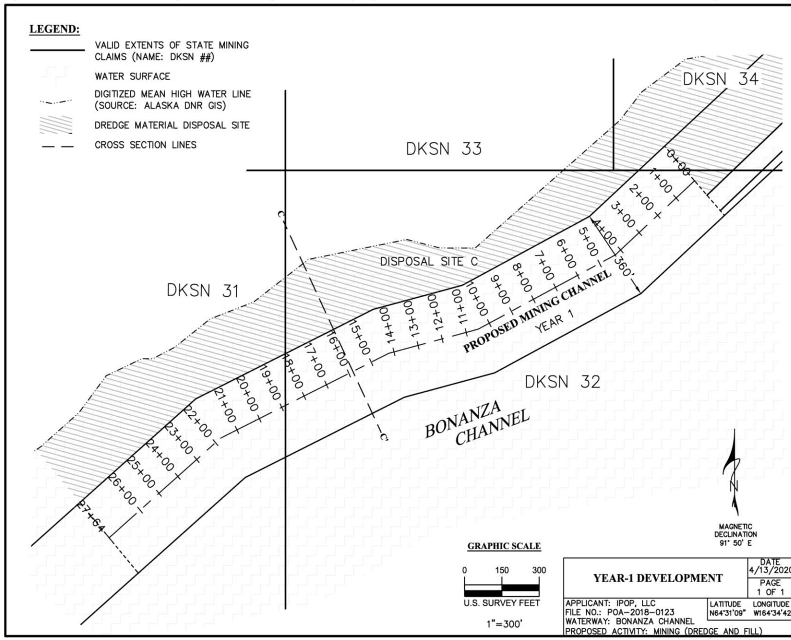
Figure 5-26. Typical dredging and filling stages (part 1) (graphic scale accurate)
