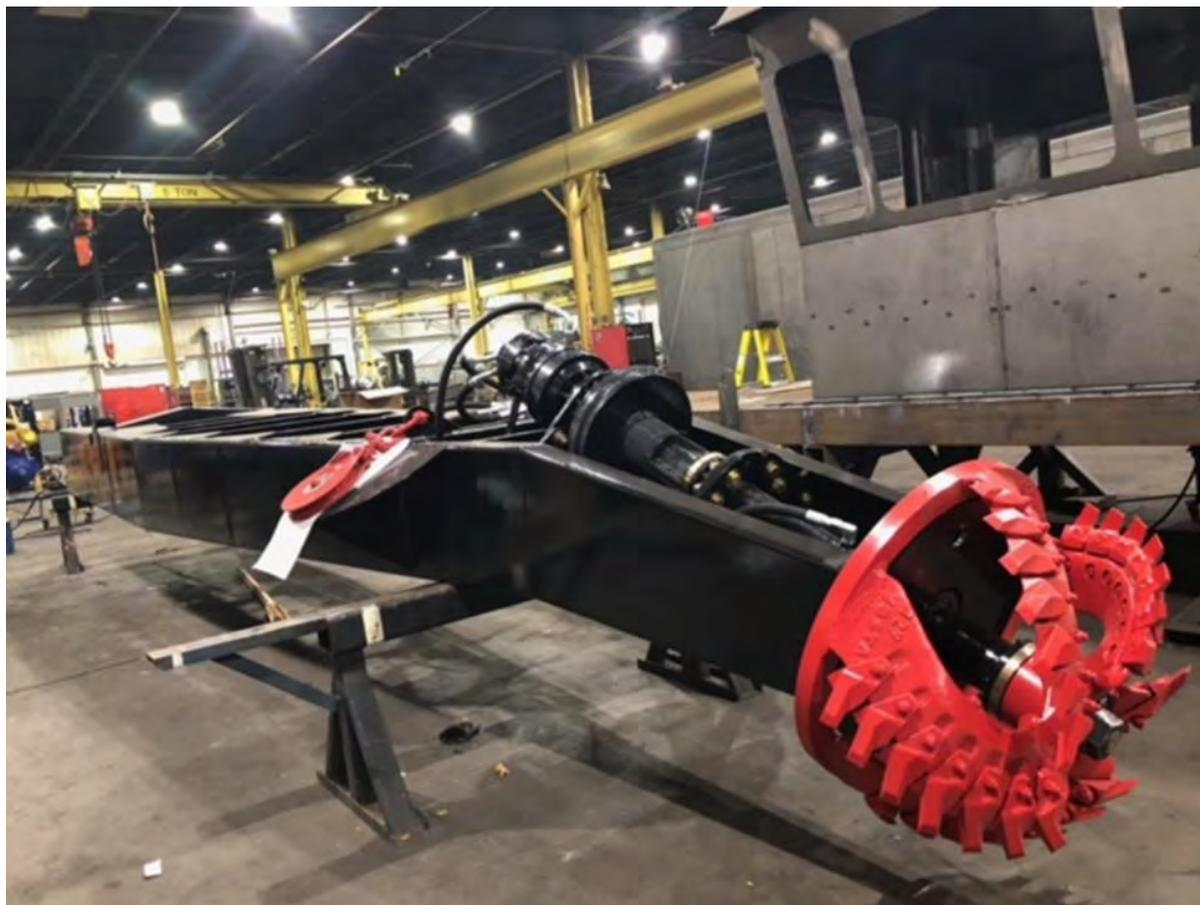
of the rear section (where it connects to the front section). The gray box on top of the barge is the power used to move the spuds.
