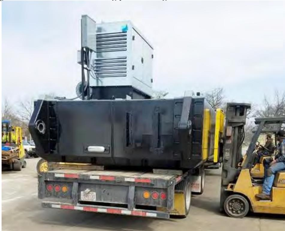
**Figure 5-10. Complete assembled cutterhead dredge and idler float**
