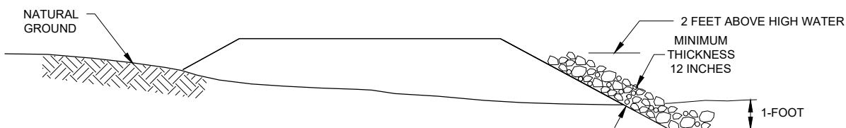
LOOSE ROCK RIPRAP USED AS SLOPE PROTECTION
