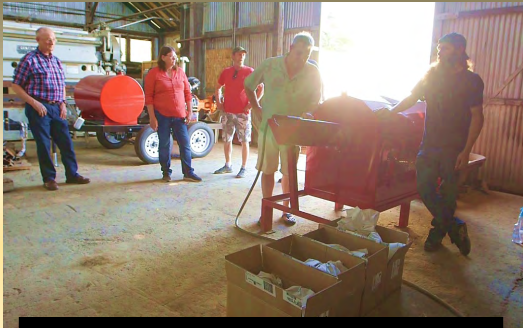
PROCESSING STARTS WITH LARGE CENTRIFUGE
