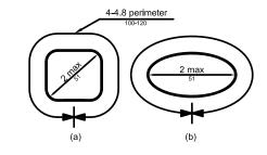
FIGURE 609.2.2 GRAB BAR NON-CIRCULAR CROSS SECTION
