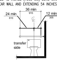
FIGURE 604.5.1 SIDE WALL GRAB BAR AT WATER CLOSEFF GURE 604.5.2 REAR WALL GRAB BAR AT WATER CLOSETS
