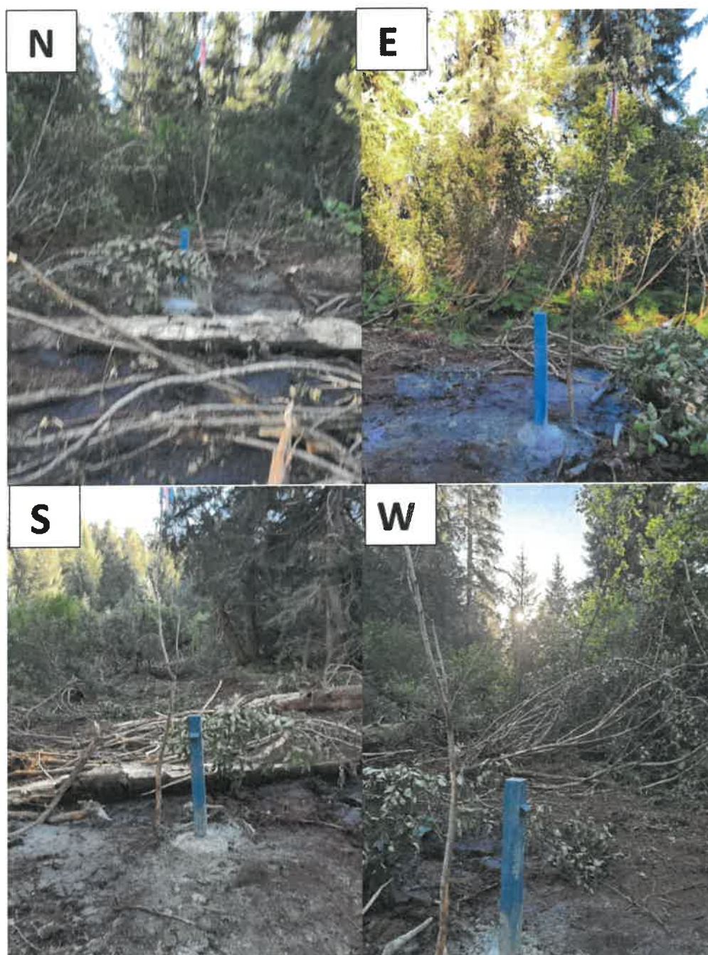
Photo 40: Overburden drillhole A2023-P1-05. A single monitoring well is capped with a protective monument.
