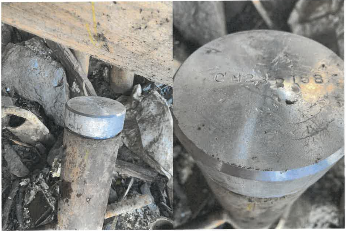
Photo 10: Stryker Pad diamond drill hole CMR23-158 is covered with removable monument and capped.
