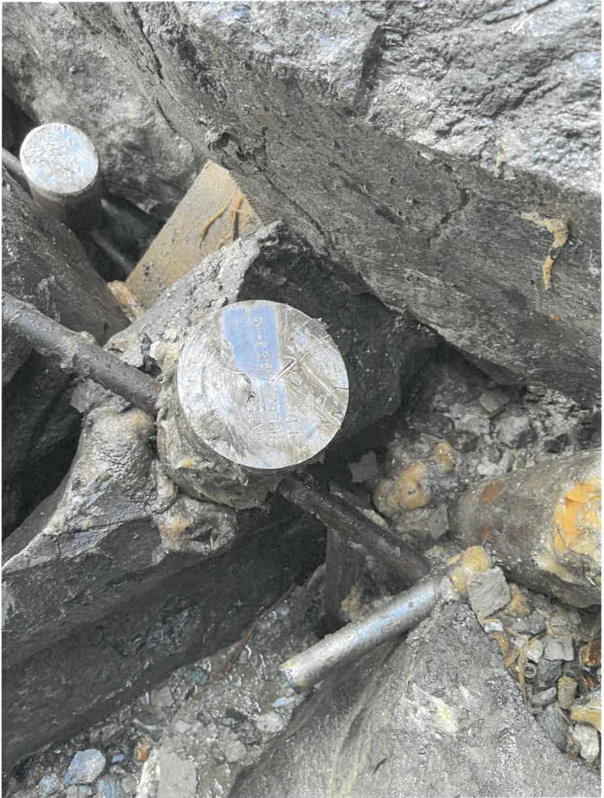
Phot 19: Merrill's Pad diamond drill hole CMR23-167 is covered with removable monument and capped.
