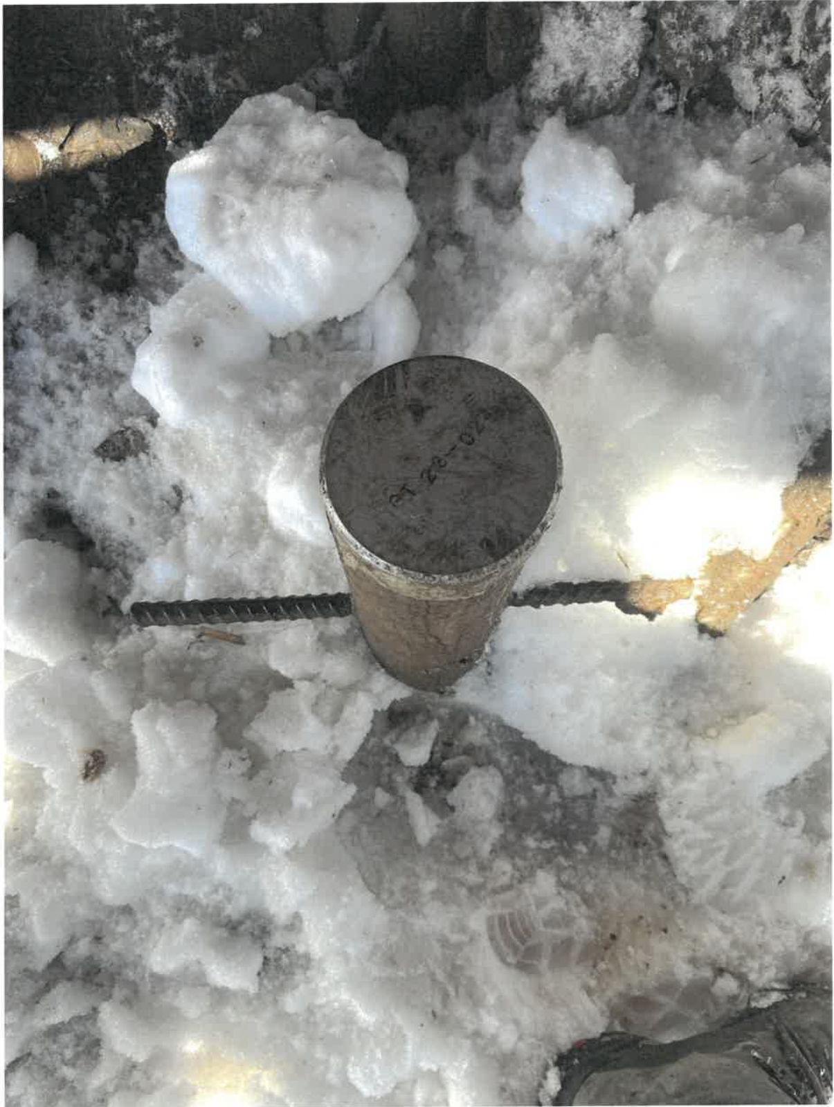
Photo 34: UM Pad diamond drill hole GT23-024 is covered with removable monument and capped.
