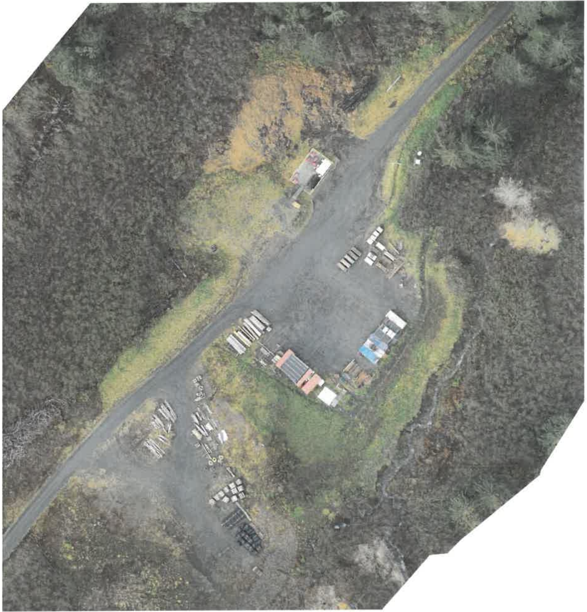
Photo 2. Glacier Creek Laydown. Six shipping containers, pallets of core boxes, some lumber, and drilling equipment (drill rods, fuel, mud tanks) are temporarily stored at the laydown. Photo is oriented north.
