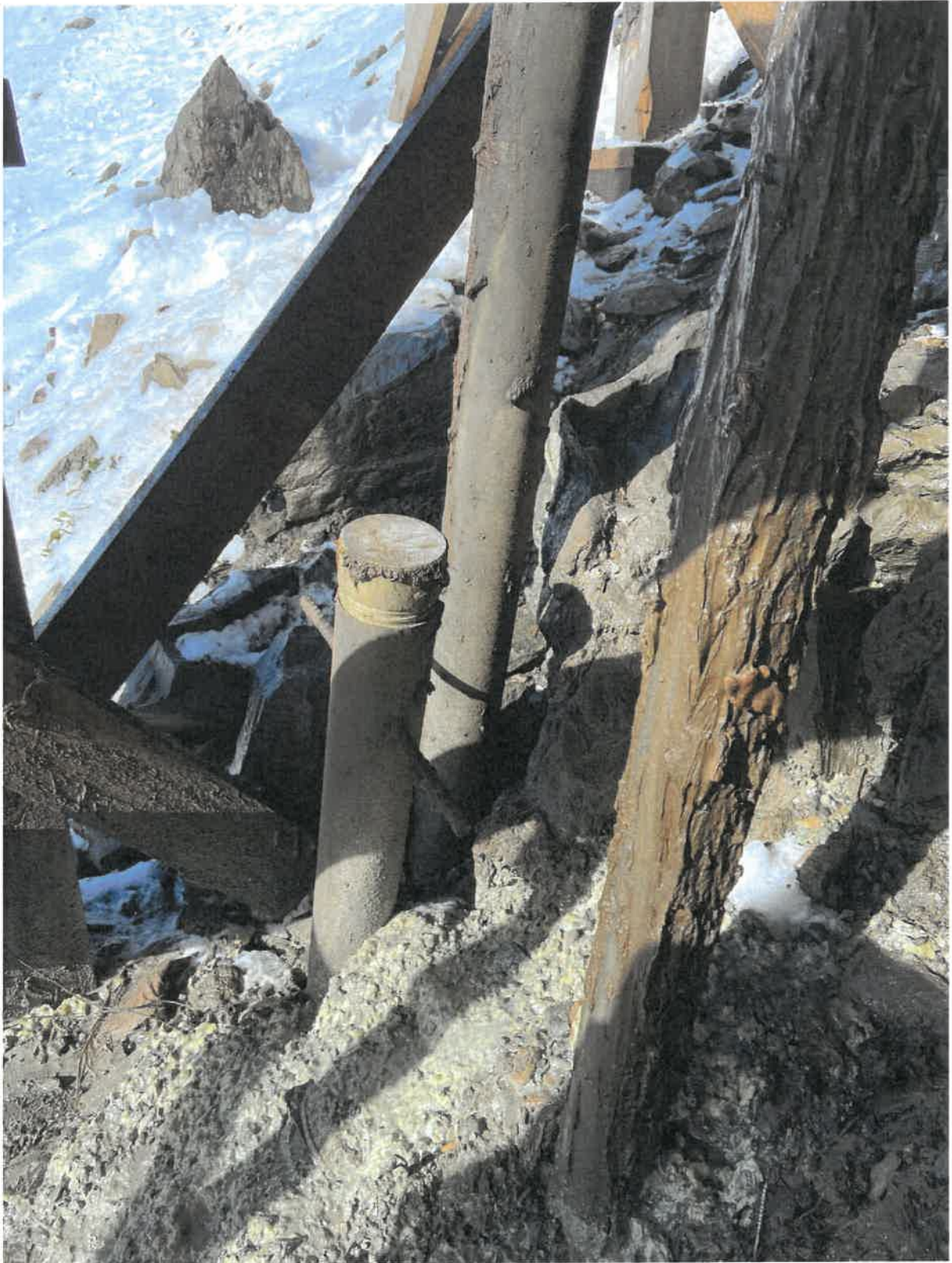
Photo 33: UM Pad diamond drill hole GT23-022 is covered with removable monument and capped.
