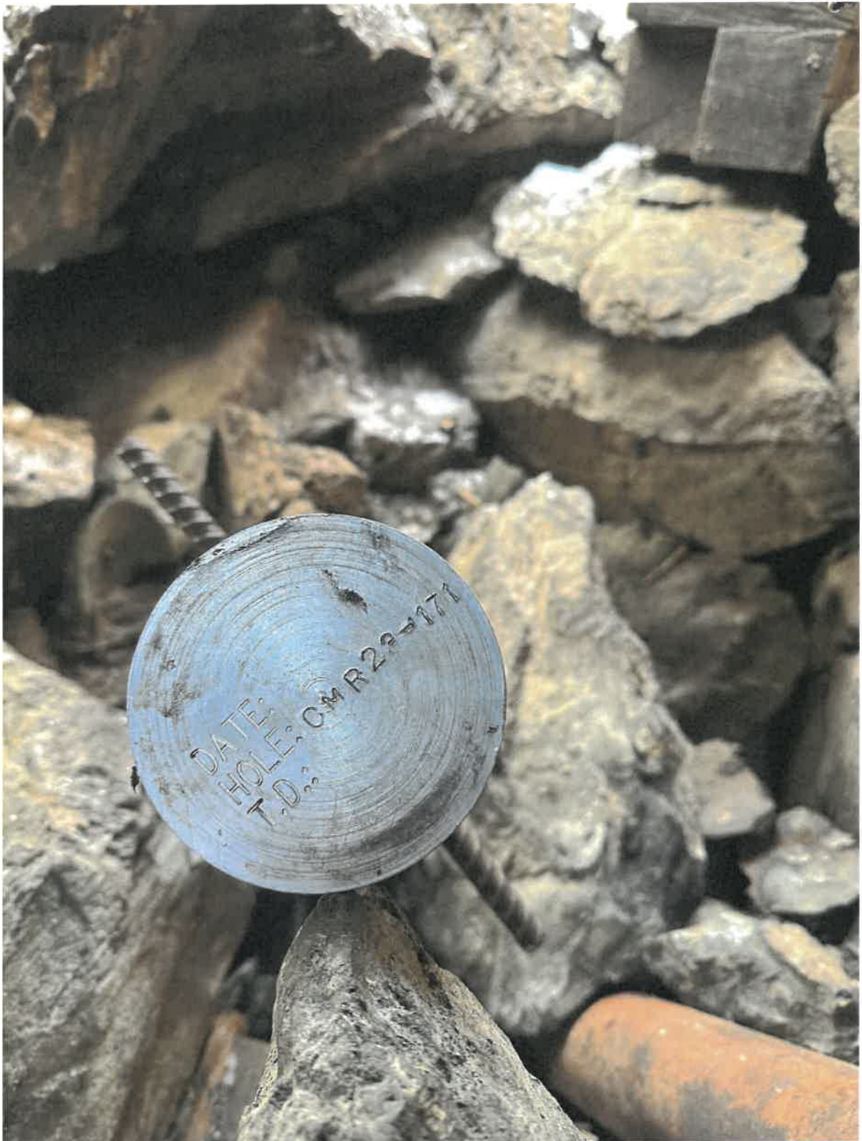
Photo 23: Merrill's Pad diamond drill CMR23-171 hole is covered with removable monument and capped.
