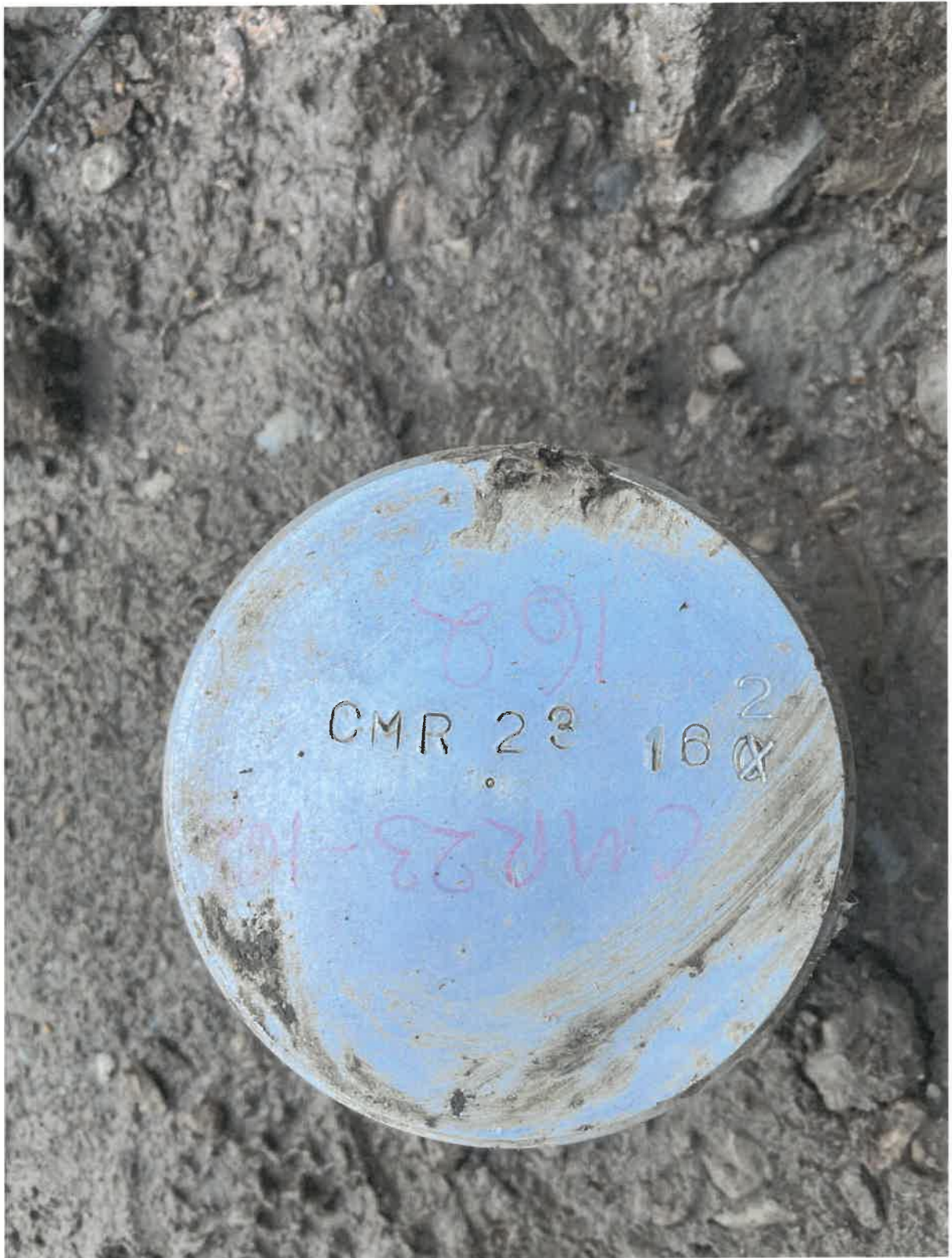
Photo 14: Stryker Pad diamond drill hole CMR23-162 is covered with removable monument and capped.
