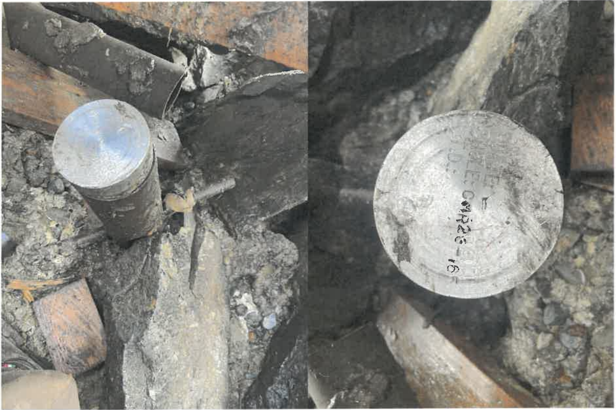
Photo 17: Merrill's Pad diamond drill hole CMR23-165 is covered with removable monument and capped.
