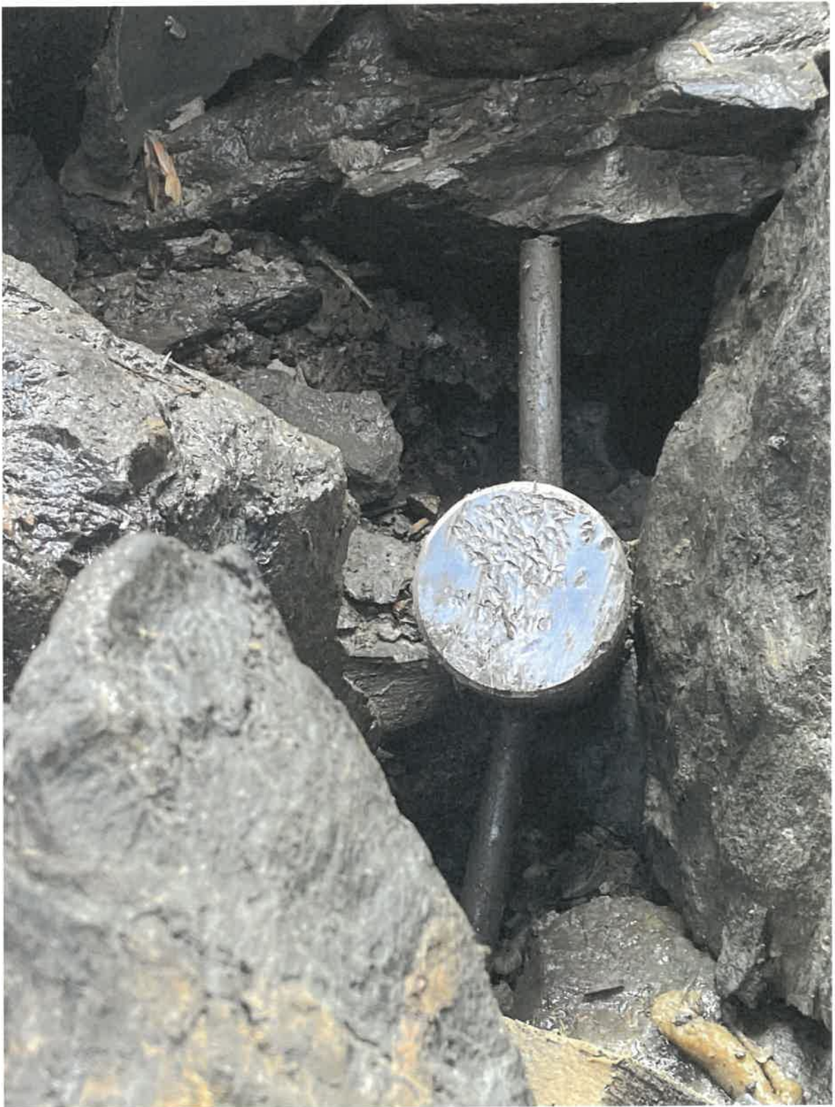
Photo 21: Merrill's Pad diamond drill hole CMR23-169 is covered with removable monument and capped.
