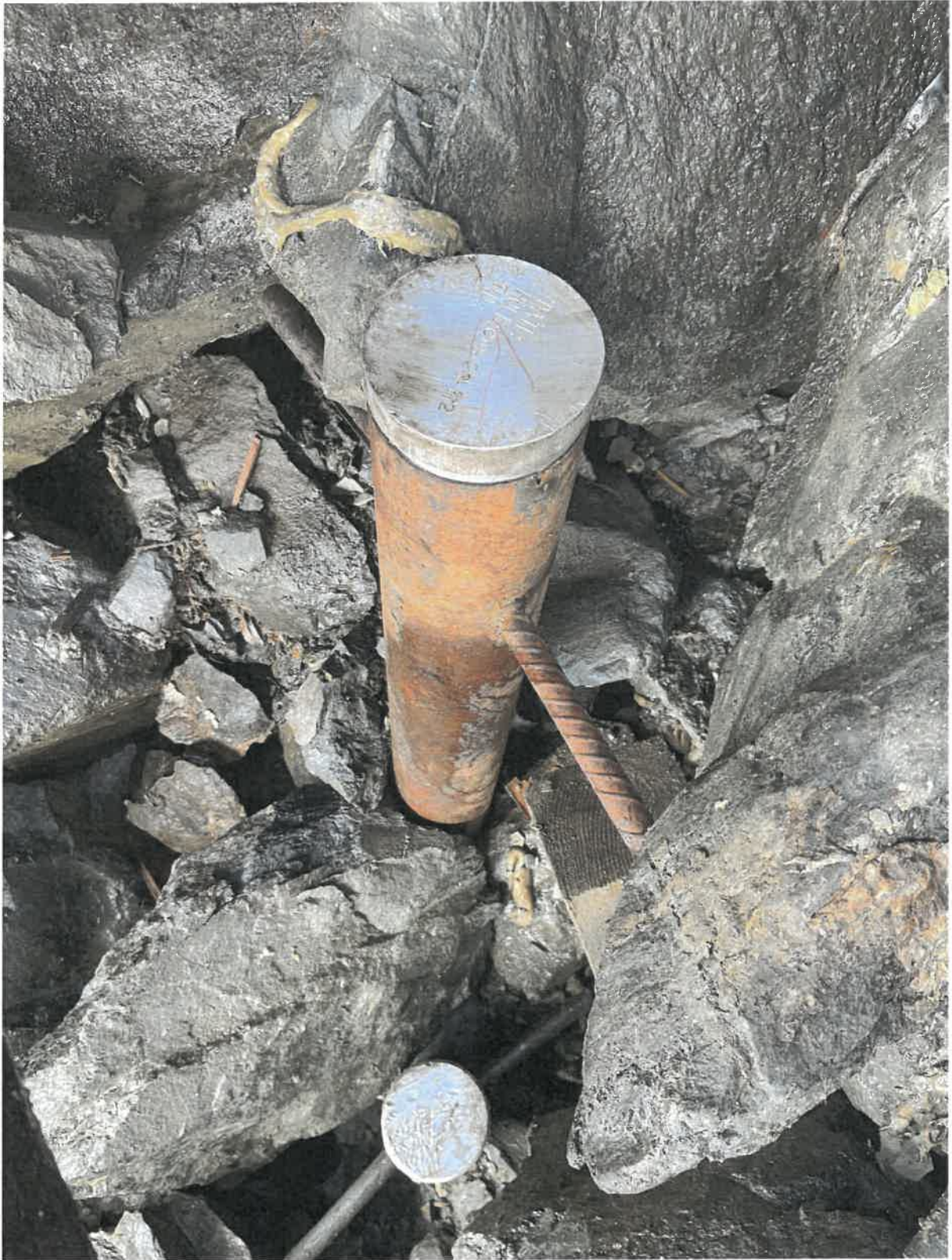
Photo 24: Merrill's Pad diamond drill hole CMR23-172 is covered with removable monument and capped.
