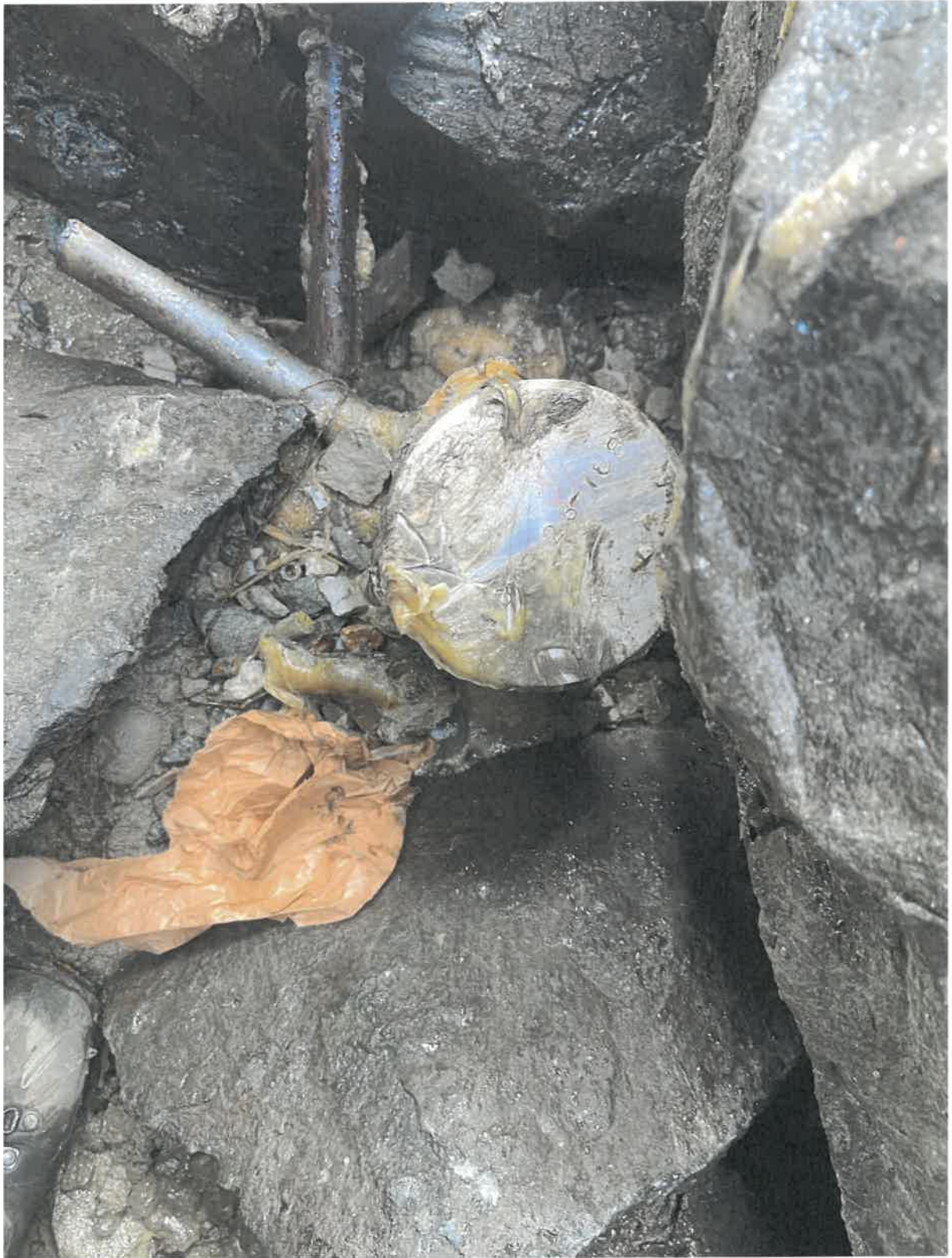
Photo 20: Merrill's Pad diamond drill hole CMR23-168 is covered with removable monument and capped.
