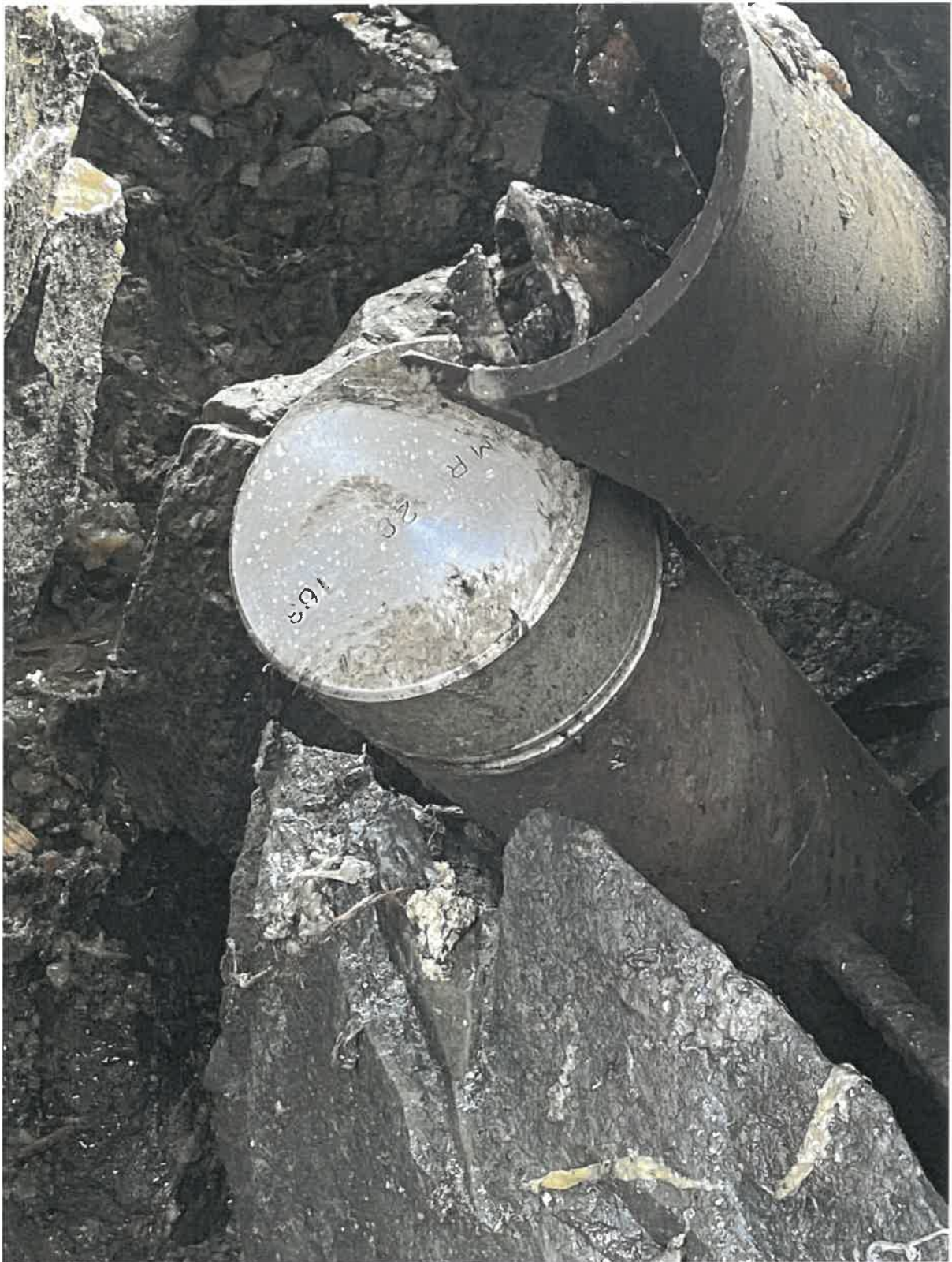
Photo 15: Merrill's Pad diamond drill hole CMR23-163/B is covered with removable monument and capped.
