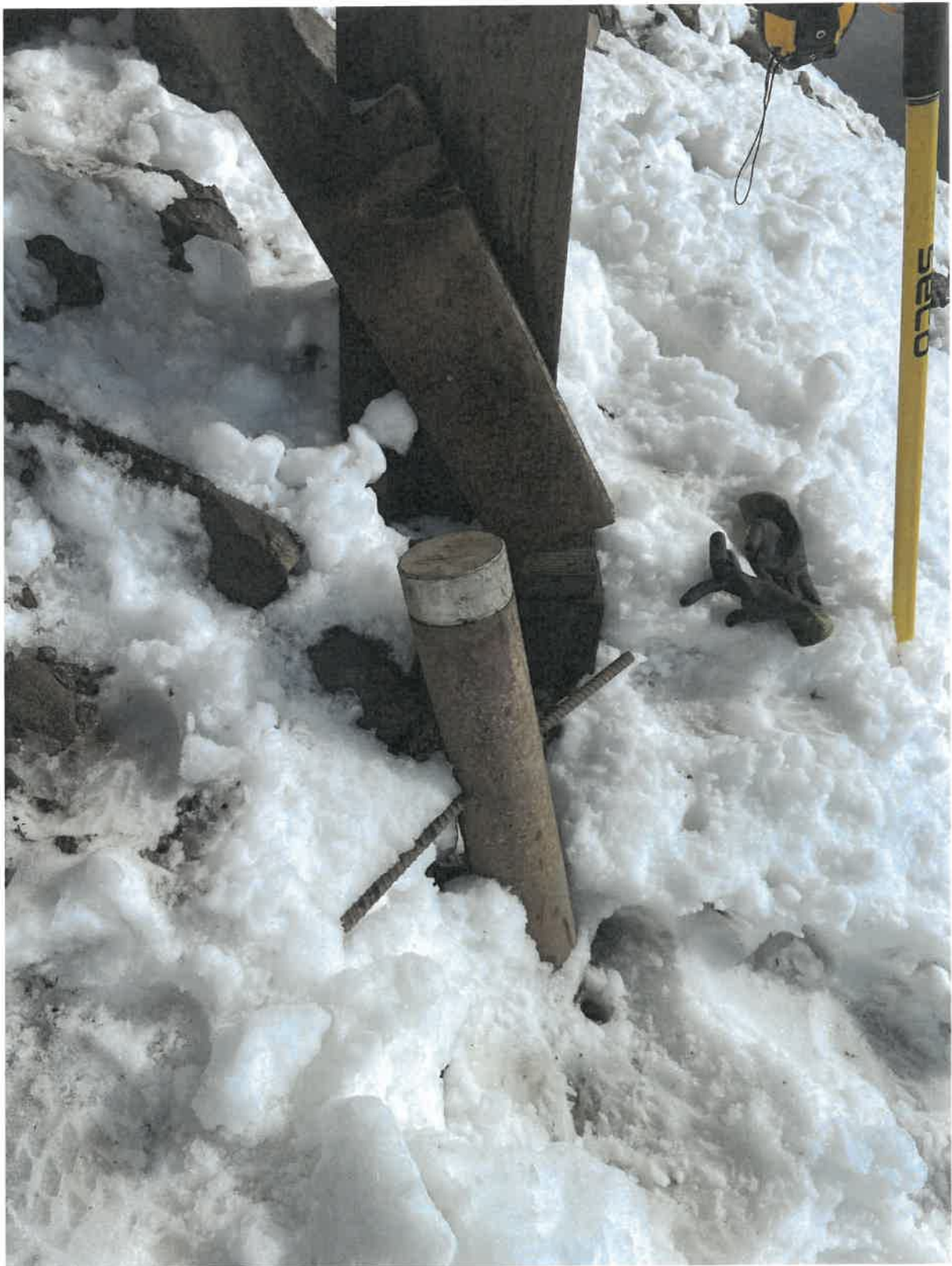
Photo 32: UM Pad diamond drill hole GT23-021 is covered with removable monument and capped.
