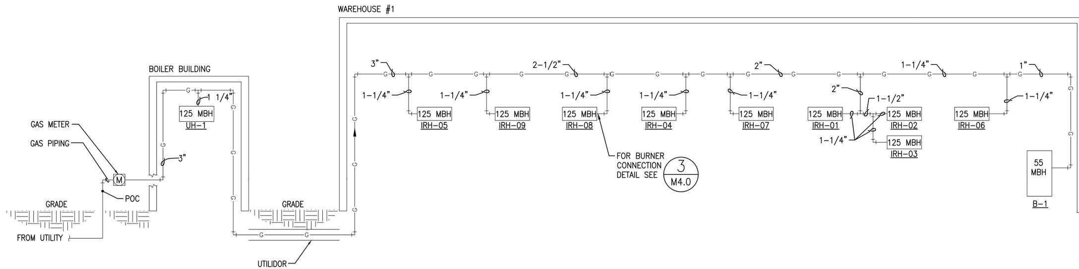
NEW GAS PIPING SERVING UH-1, IRH-1 THRU 9, AND B-1
