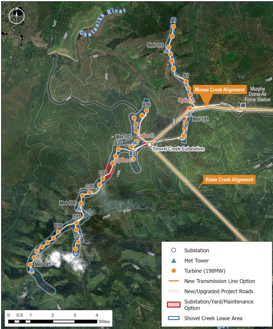
Figure 3. Detailed map of the project area indicating potential substation, yard, and maintenance building parcel locations as well as turbine layouts optimized based on recent meteorological data.
