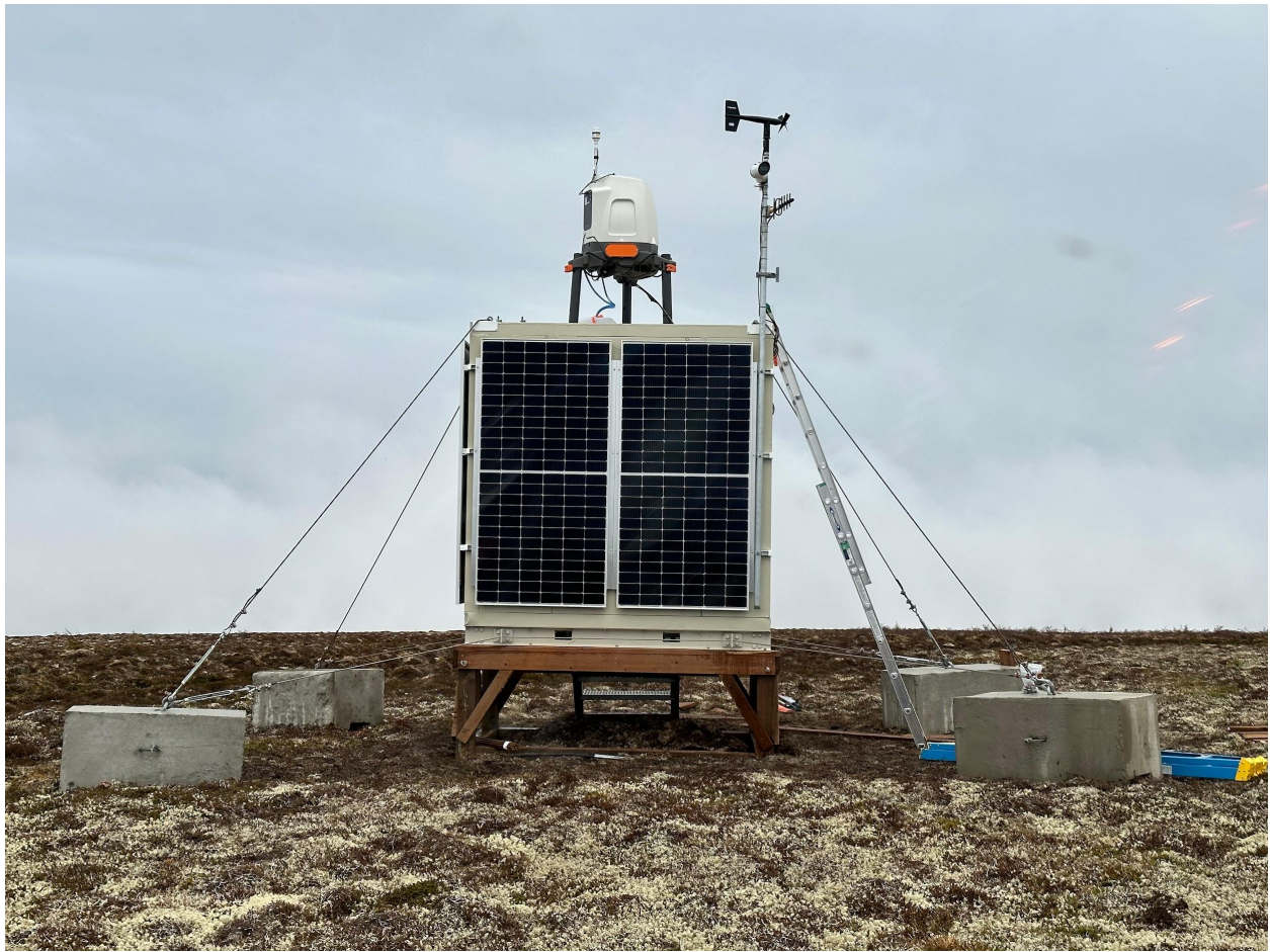
Example of a remote power supply unit and roof-mounted Lidar system.
