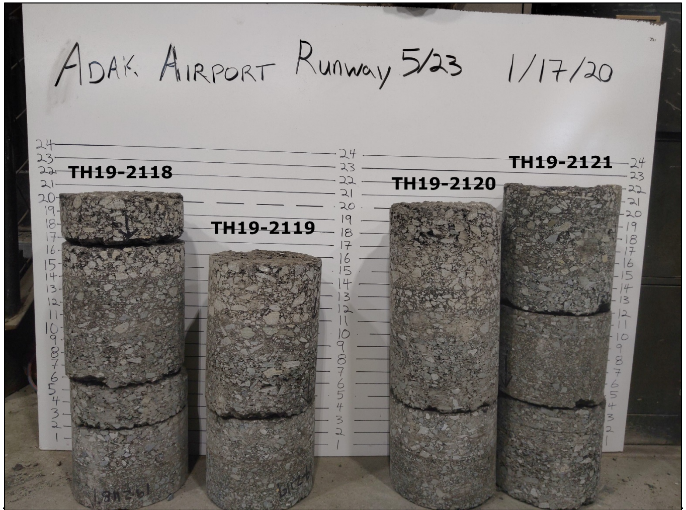
Photo 7: Runway 5/23 Asphalt Cores
