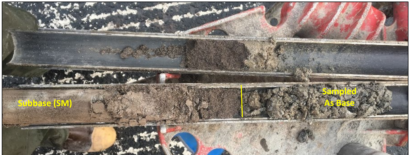
Photo 9: Sample 19-9023 from test hole TH19-2107 depths 15-39" (below asphalt) showing the subbase, silty sand (SM). Base course consists of silty sand with gravel.
