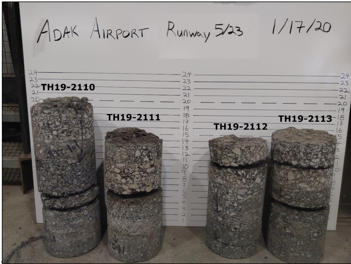
Photo 5: Runway 5/23 Asphalt Cores
