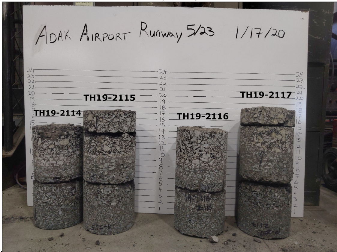
Photo 6: Runway 5/23 Asphalt Cores
