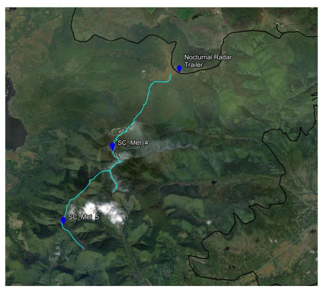
Light blue line indicates the proposed access trail that departs towards the SW from an existing trail in the vicinity of Murphy Dome Extension Rd (black line at top). SC\_Met\_4 and SC\_Met\_5 are the proposed meteorological tower and lidar remote sensing sites.
