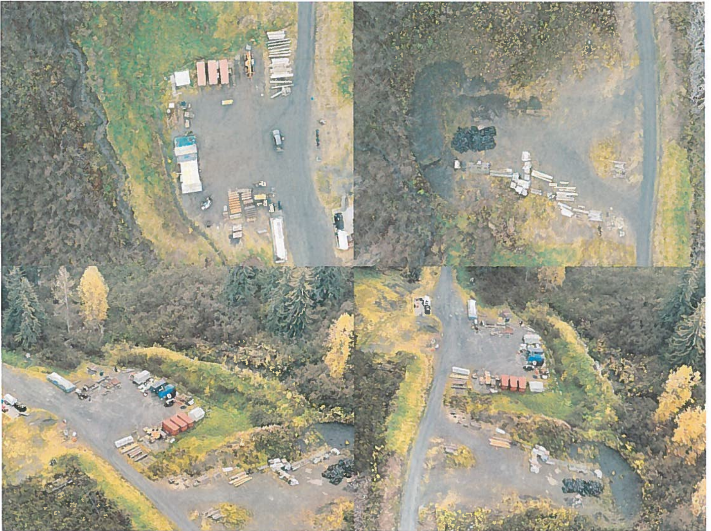
Photo 3. Glacier Creek Laydown. Six shipping containers, pallets of core boxes, some lumber, and drilling equipment (drill rods, fuel, mud tanks) are temporarily stored at the laydown (Photo: Oct 2022).
