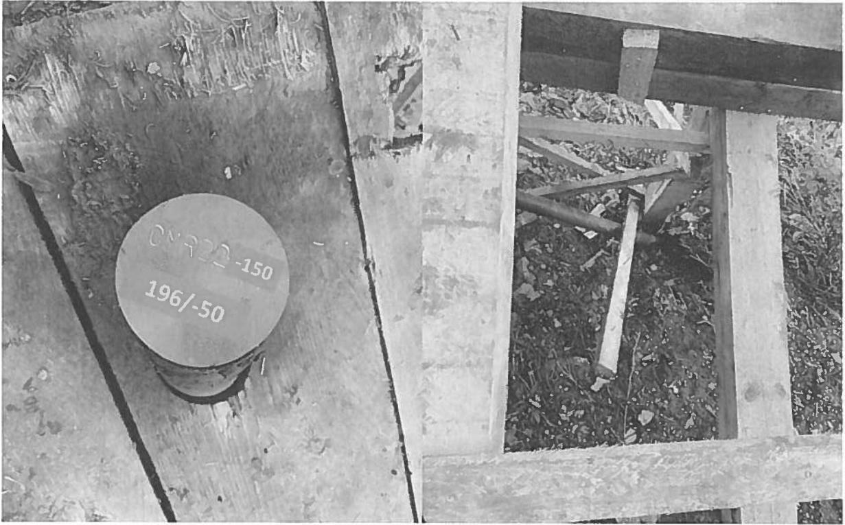
Photo 9: Hari Pad diamond drill hole CMR22-150 is capped for future re-entrance.
