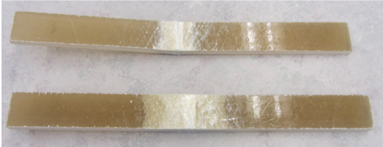
Fig. 4 Failed samples under the 3-point bending tests
