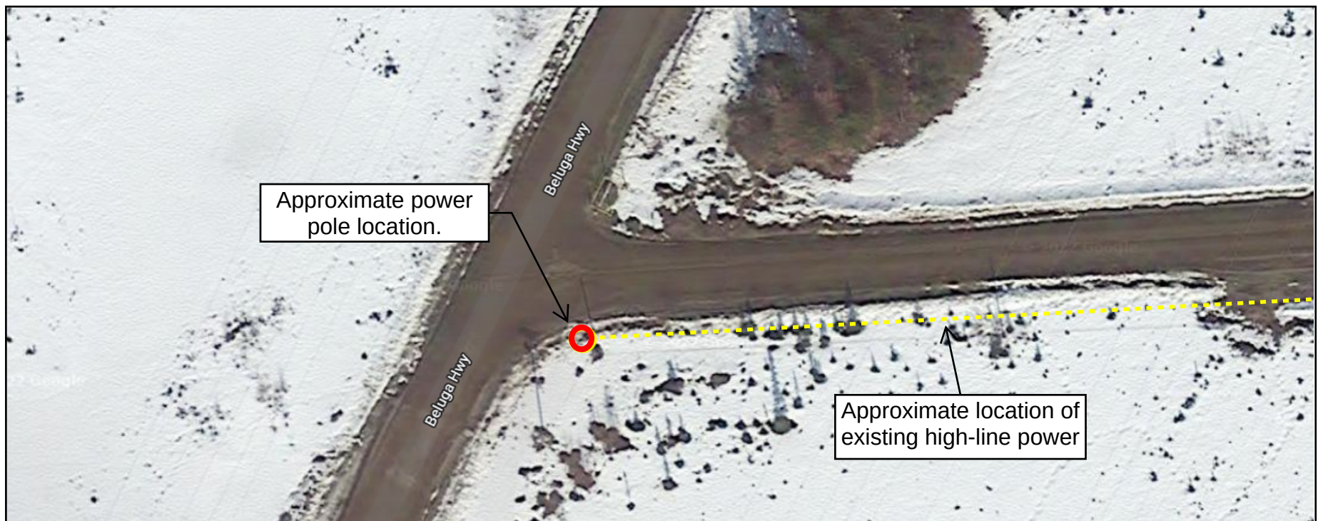
Approximate location of power pole at the entrance of K-Pad. Installation will require an approximate 5-6 foot excavation.
