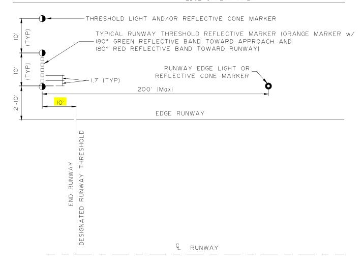
Figure 660-1 Typical Threshold Detail No Scale
