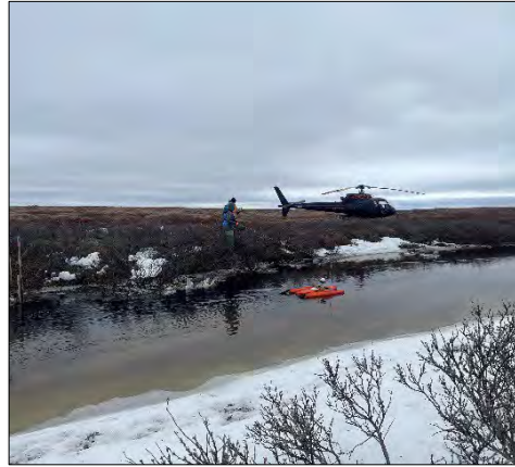
Photograph 11. Tethered Acoustic Doppler current profilers.
