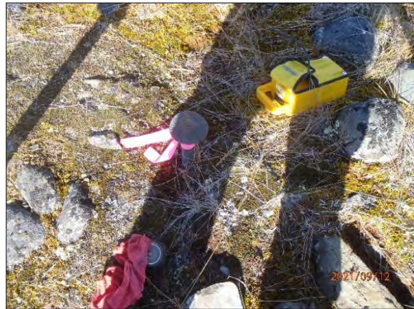
Photograph 16. Example of primary control monument (post monument with cap).
