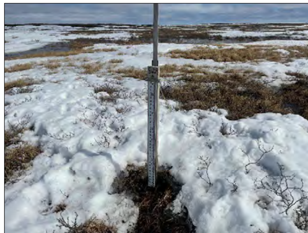
Photograph 12. Staff gage mounted on T-post driven into ground.
