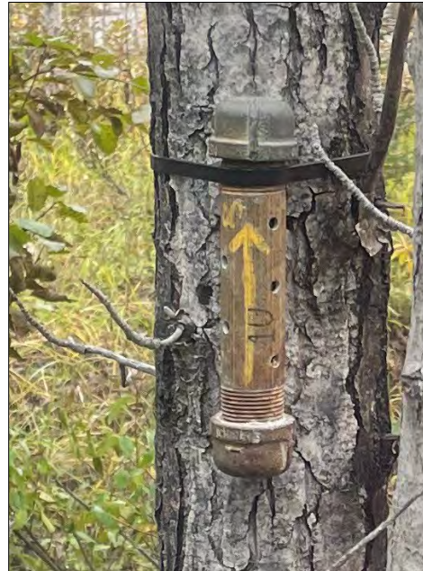
Photograph 9. Pressure sensor anchored to tree.
