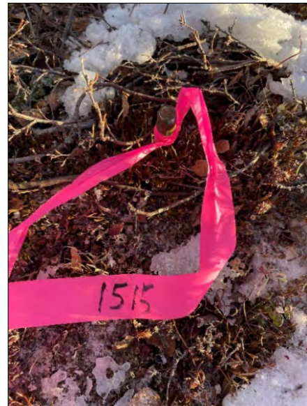
Photograph 18. Example of secondary control monument (rebar with aluminum cap).
