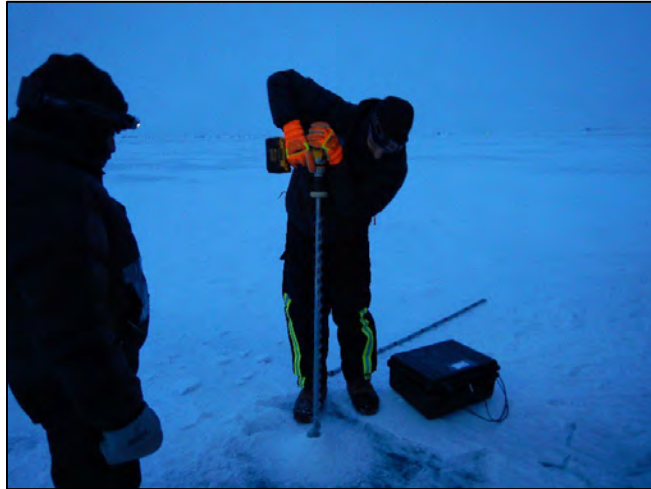
Photograph 7. Drilling through ice using a 2-inch auger.
