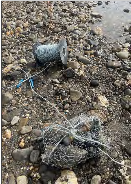
Photograph 8. Pressure sensor anchored using weight.
