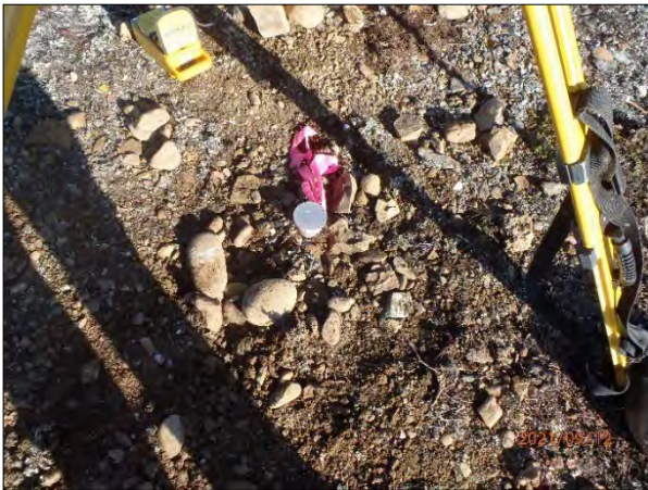
Photograph 15. Example of primary control monument (brass tablet grouted into bedrock).
