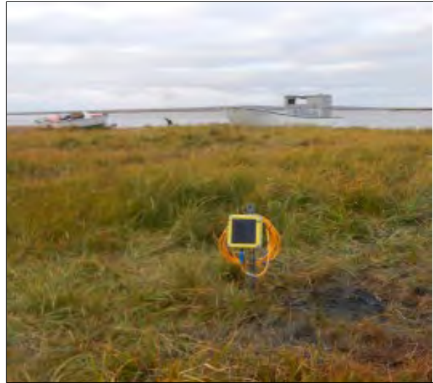
Photograph 29. Example of installed thermistor well, DTC, and datalogger.
