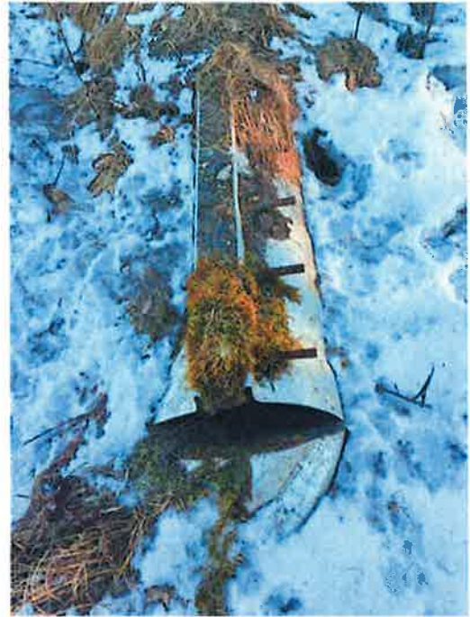
Sewer service line separating at the 45 joint - a common issue in the Pilcher View Subdivision.
