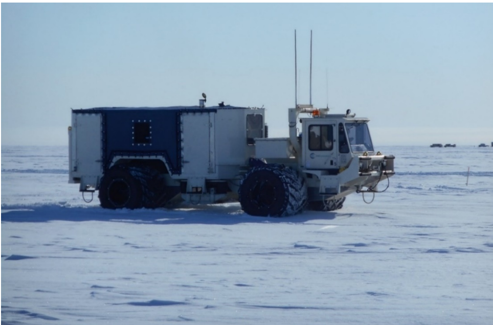
Photo 3: AHV4 Commander Vibrator (Source Equipment) Approx. 60,000 pounds with tires
