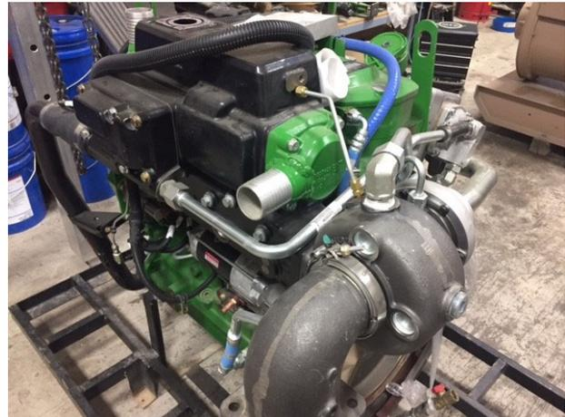
2. 6068AFM - Remove coolant tank and other accessories that are not required. Modify coolant discharge and suction connections to face horizontally at the front of the engine using bent steel tubing and short sections of silicone hose. Support steel tube from skid and engine. See photograph below for representative installation.
