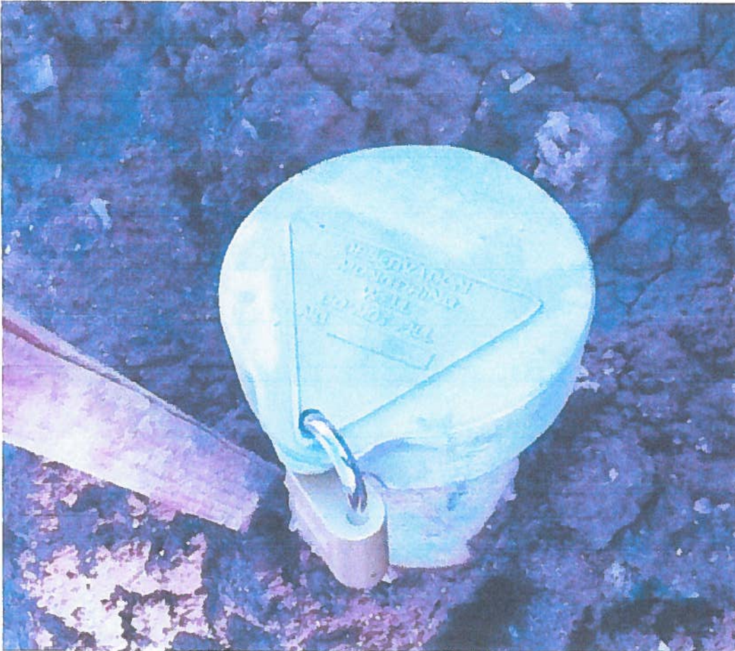
Photograph of closed drill hole AM20-01 capped and locked on drill pad 1 from the Amanita 2020 drilling. This drill hole had standing water and will be used as a temporary water source for drilling during the 2021-2025 exploration.
