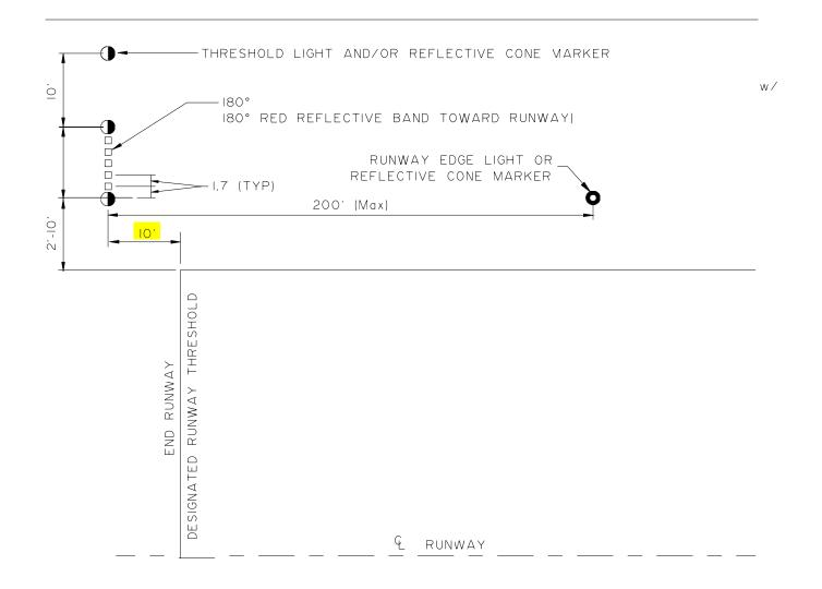
Figure 660-1 Typical Threshold Detail No Scale
