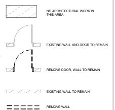
KEYNOTES () REMOVE MATERIALS NOT REUSED IN NEW CONSTRUCTION. THIS INCLUDES INTERIOR WALLS, CASEWORK, FIXTURES, DOORS AND WALL MOUNTED ITEMS, FLOOR MOUNTED ITEMS, AND CEILING MOUNTED ITEMS; UNLESS OTHERWISE INDICATED.
