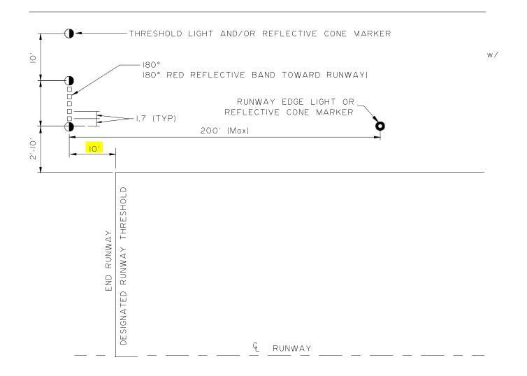
Figure 660-1 Typical Threshold Detail No Scale
